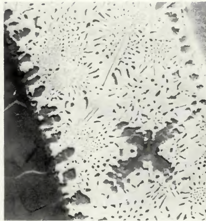
Fig. 21—A (left)—normal structure in some regions of Skylab nickel specimens and all ground-brazed specimens; B (right)—abnormal structure seen in other regions of the Skylab specimens. \times 500 (reduced 28% on reproduction)
