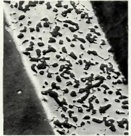
Fig. 21—A (left)—normal structure in some regions of Skylab nickel specimens and all ground-brazed specimens; B (right)—abnormal structure seen in other regions of the Skylab specimens. \times 500 (reduced 28% on reproduction)
