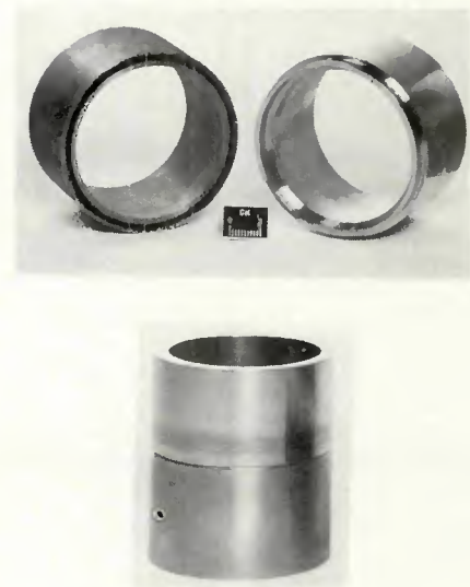
Fig. 9—Dissimilar metal pipe brazement and component parts for Hastelloy X tongue in Cb-1Zr groove
