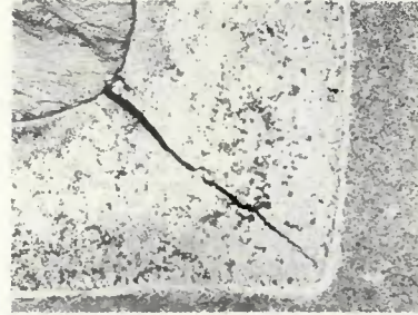
(b) Local cracks in as-brazed BNi-4 joint at tip of tongue.
