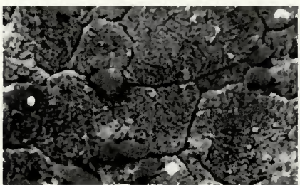
Fig. 6—Scanning electron micrograph showing grooving of brazing alloy after 4 min at 550 C in a vacuum of 10^{-3} torr (133 mPa). \times 2000 (reduced by 33% on reproduction)
