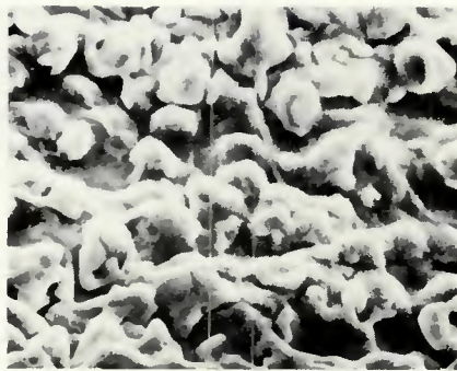
Fig. 13—Scanning electron micrograph of new surface formed on brazing sheet heated at 560 C in a vacuum of 5 \times 10^{-3} torr (6.7 mPa). \times 1000 (reduced by 33% on reproduction)
