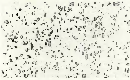
Fig. 2—Unetched surface of brazing alloy after 4 min at 510 C in vacuum. \times 500 (reduced by 33% on reproduction)
