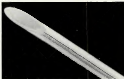
Fig. 1—The composite brazing filler metal wire consists of a powder core, which is tightly enclosed by a metal sheath
