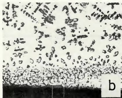
Fig. 7—Transverse cross section through a standard composite brazing wire, the tip of which had been melted in an acetylene torch. \times 9 (reduced by 28% on reproduction)
