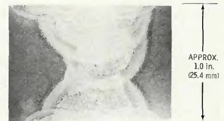
Fig. 2—Macrograph of type 2 weld; nital etch
