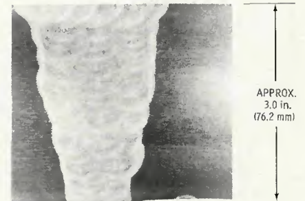
Fig. 1—Macrograph of type 1 weld; nital etch
