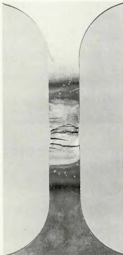
Fig. 12—Cracks in a 4340 steel specimen which has been GMA surfaced with Cu while under a 16 ksi stress. Cu has been chemically removed. 2X (reduced 50% to original size during printing reproduction)
