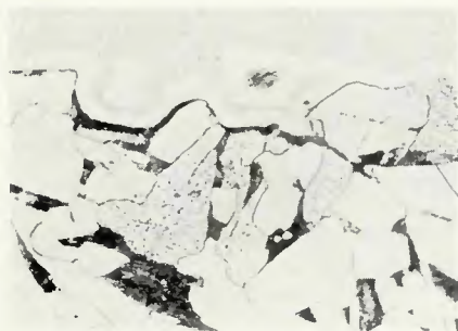
Fig. 9—Photomicrograph of 1026 steel after furnace-brazing exposure to Cu for 2 h at 2050 F. Nital etch, X500 (reduced 50% during printing reproduction)
