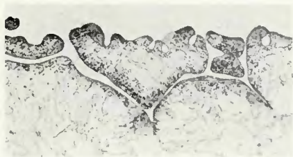
Fig. 8—Photomicrograph of decarburized 4340 steel after furnace-brazing exposure to Cu for 2 h at 2050 F. Nital etch, X500 (reduced 59% during printing reproduction)
