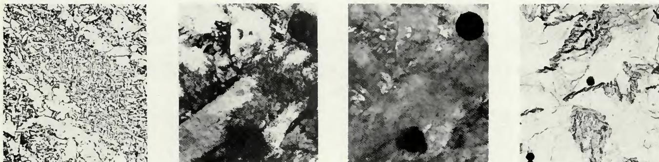
Fig. 3—Weld metal of 1.4% Mn. From left: A—light micrograph; B—transmission bright field; C—dark field; D—replica. A— $\times 500$ ; B, C and D— $\times 50,000$  (reduced 31% on reproduction)
