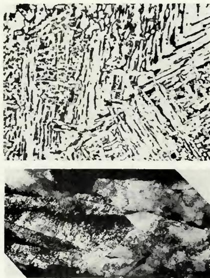
Fig. 4—Lath type structure found in the 2.2% Mn weld metal: A (top)—light micrograph; B (bottom)—electron micrograph. A— $\times 500$  (no reduction); B— $\times 65,000$  (reduced 57% on reproduction)
