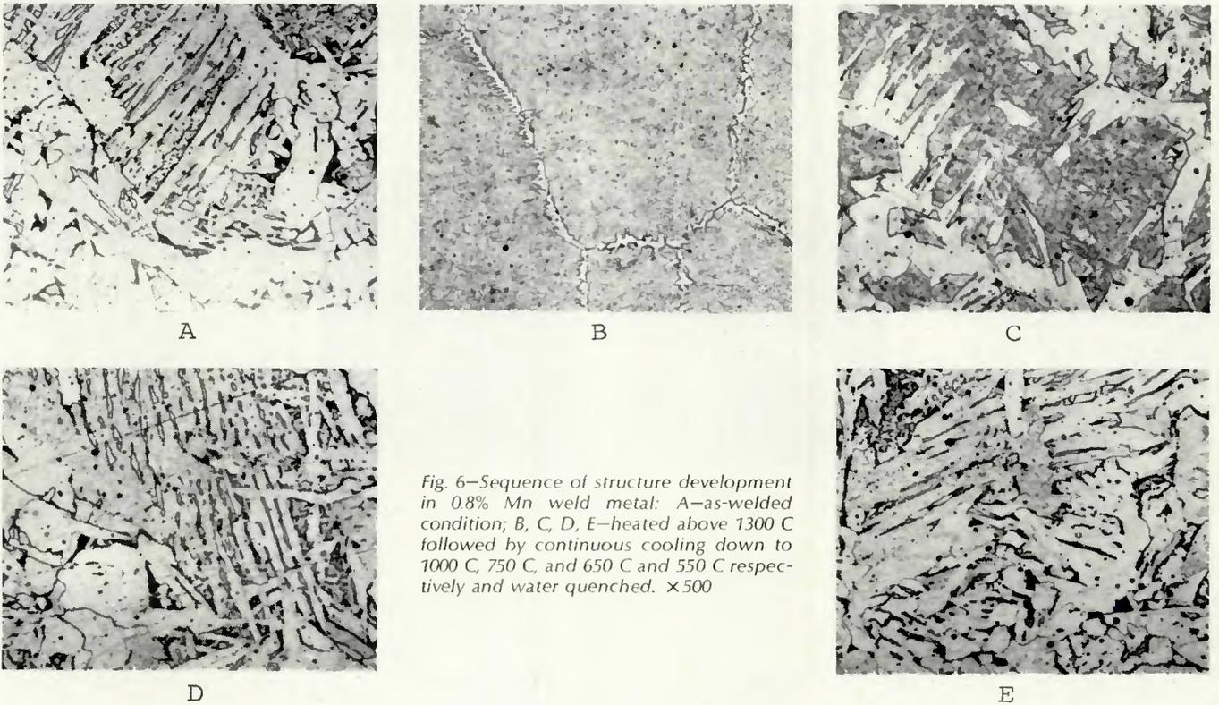
Fig. 6—Sequence of structure development in 0.8% Mn weld metal: A—*as-welded condition*; B, C, D, E—*heated above 1300 C followed by continuous cooling down to 1000 C, 750 C, and 650 C and 550 C respectively and water quenched.*  $\times 500$
