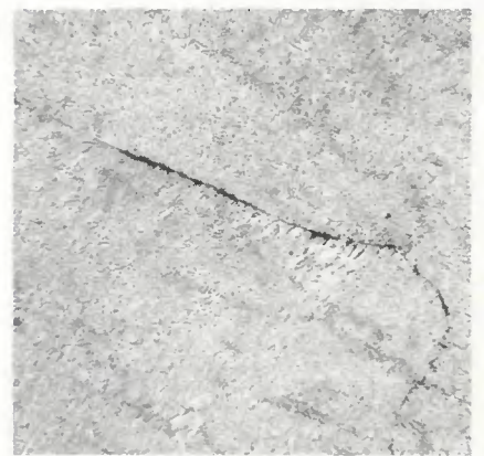
Fig. 4—Microstructure and grain boundary crack in the weld metal from electrode L100. 2% nital etch; X100 (reduced 28% on reproduction)
