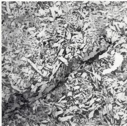
Fig. 1—Microstructure and grain boundary crack in the weld metal from electrode L36. 2% nital etch; X100 (reduced 28% on reproduction)
