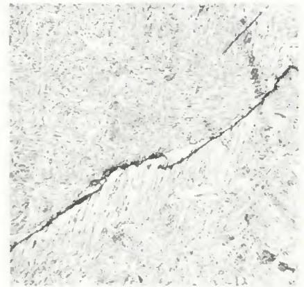
Fig. 3—Microstructure and grain boundary crack in the weld metal from electrode AW19. 2% nital etch; X100 (reduced 28% on reproduction)
