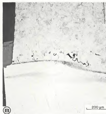
Fig. 7—Cracks formed in specimen tested at 138 MPA at 593°C (1099°F) for 2300 h and 64 cycles. Before test, specimen was tempered 10 h at 732°C (1350°F). A—unetched; B—etched in 2% nital
