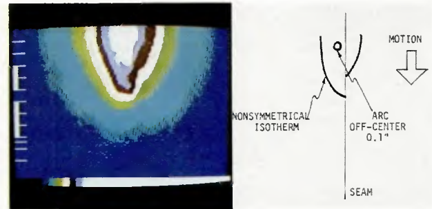
Fig. 14—Nonsymmetric moving arc temperature distribution. Arc traversing down the joint, 0.1 in. (2.5 mm) off-center
