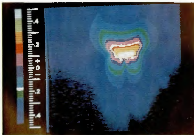
Fig. 15—Effect of plate gaps on moving arc temperature distribution. The plate gap is indicated by the notches in the color boundaries (isotherms). Note how far ahead of the arc the gap can be detected
