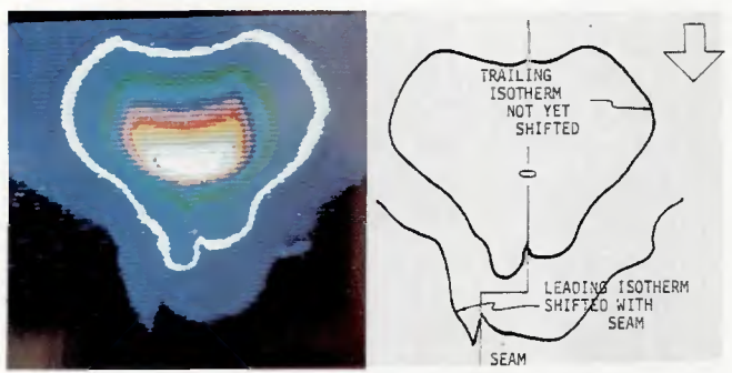
Fig. 17—Seam tracking—shifted portion. The leading isotherm indicates the upcoming shift in the joint. This demonstrates that impending tracking errors can be detected
