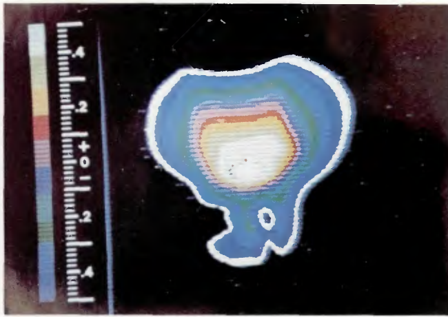
Fig. 18—Impurities in a moving arc. The small white circle indicates a cold spot ahead of the arc. This was caused by an impurity placed in the weld path
