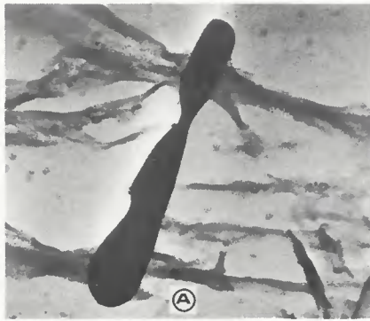
Fig. 4—Irregular shaped inclusions associated with: A—code H flux; B—code D flux. \times 11000 (reduced 50% on reproduction)
