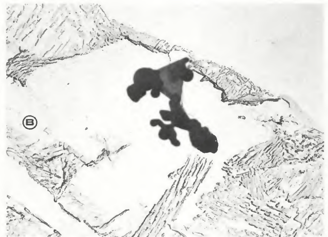
Fig. 5—Duplex nature of irregular shaped inclusions associated with: A—code C flux; B—code E flux. Magnifications as follows: A— \times 11000 ; B— \times 15000 (reduced 44% on reproduction)
