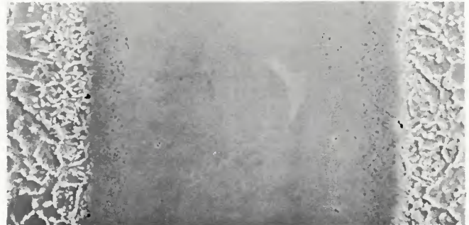
Fig. 6—SEM photomicrograph of joint brazed for 120 min at 1000°C (1832°F). Filler metal—NiPd-1; base metal—Type 347 stainless steel. Joint clearance—100 μm (0.004 in.); X600 (reduced 50% on reproduction)
