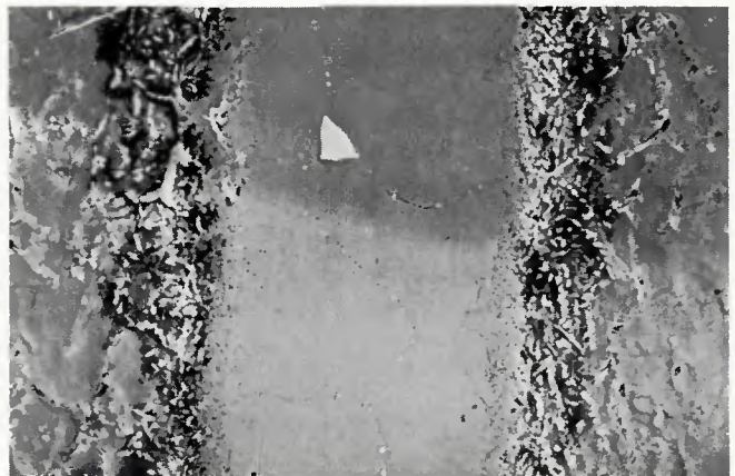
Fig. 8—SEM photomicrograph of joint brazed for 60 min at 1000°C (1832°F). Filler metal—NiAu-2; base metal—Type 347 stainless steel. Joint clearance—50 μm (0.002 in.); X600 (reduced 50% on reproduction)
