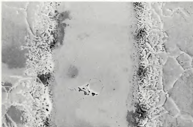
Fig. 7—SEM photomicrograph of joint brazed for 60 min at 1000°C (1832°F). Filler metal—NiPd-2; base metal—Type 347 stainless steel. Joint clearance—50 μm (0.002 in.); X600 (reduced 50% on reproduction)
