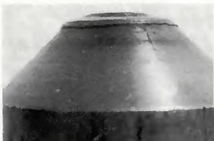
Fig. 14—Electrode deterioration—0.25 in. (6.35 mm) diameter flat face, 45 deg truncated electrode after 1500 welds
