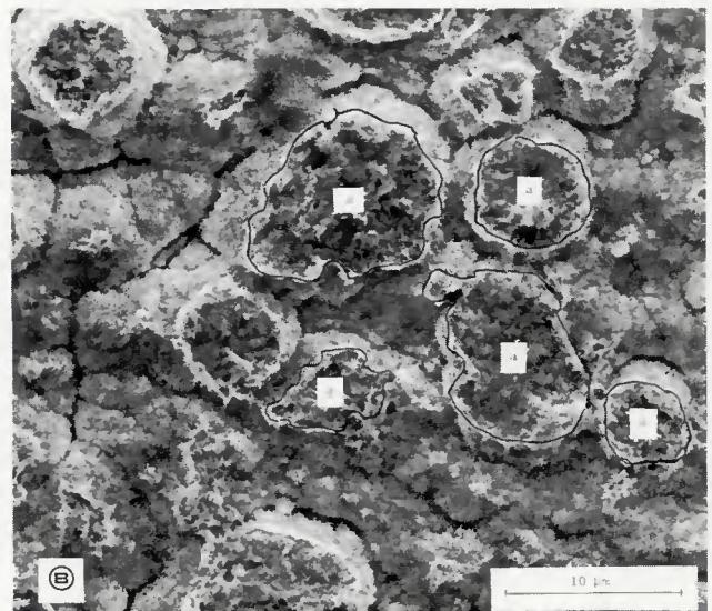
Fig. 12—Fracture surfaces of unaged welds: A—between stainless steel and pure aluminum; B—between stainless steel and 6061 aluminum alloy
