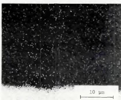
Fig. 4—Concentration distribution of Al at an unaged weld between stainless steel and 6061 aluminum alloy
