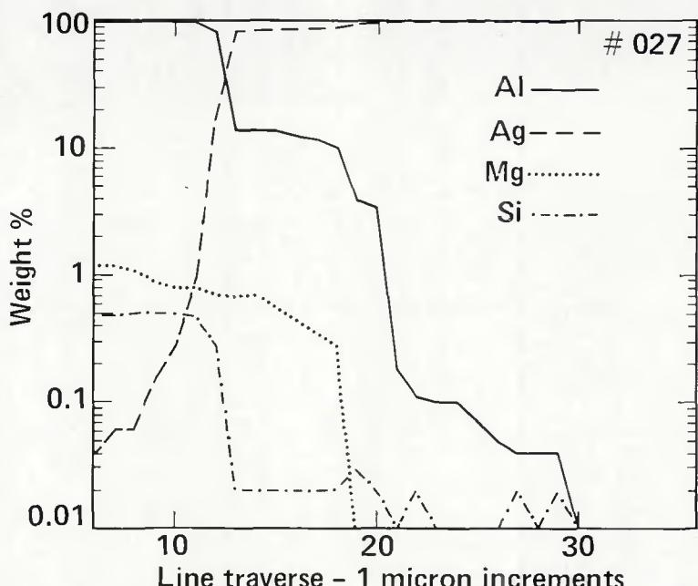
Fig. 9—Logarithmic concentration profiles at a silver/6061 aluminum alloy weld interface; specimen aged at 513 K for 49 h
