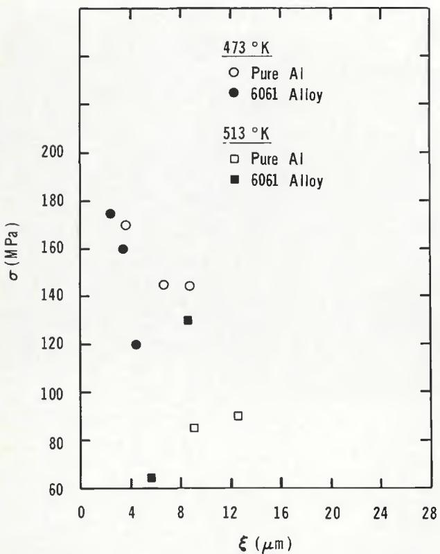
Fig. 11—The dependence of the strength of welds between stainless steel and pure aluminum and 6061 aluminum alloy on the thickness of the intermetallic layer
