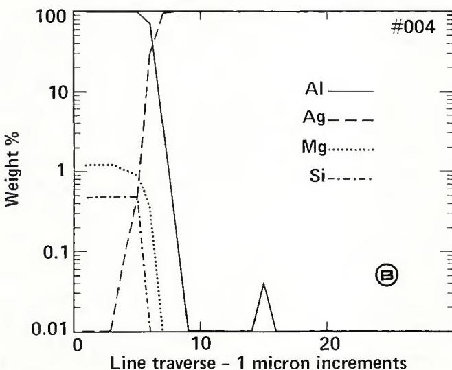
Fig. 7—Linear concentration profiles at a silver/6061 aluminum alloy weld interface; as-welded condition. A—linear concentration profile; B—logarithmic concentration profile
