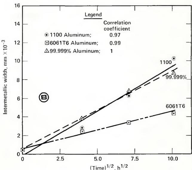
Fig. 2—The time dependence of the growth of the intermetallic layer:
