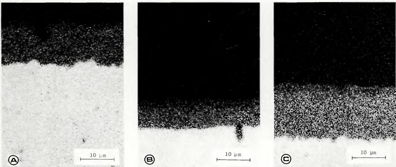
Fig. 5—X-ray maps showing aluminum distribution in welds with stainless steel after aging at 513 K for 49 h. Welds made as follows: A—With pure aluminum; B—with 6061 aluminum alloy; C—with 1100 aluminum alloy
