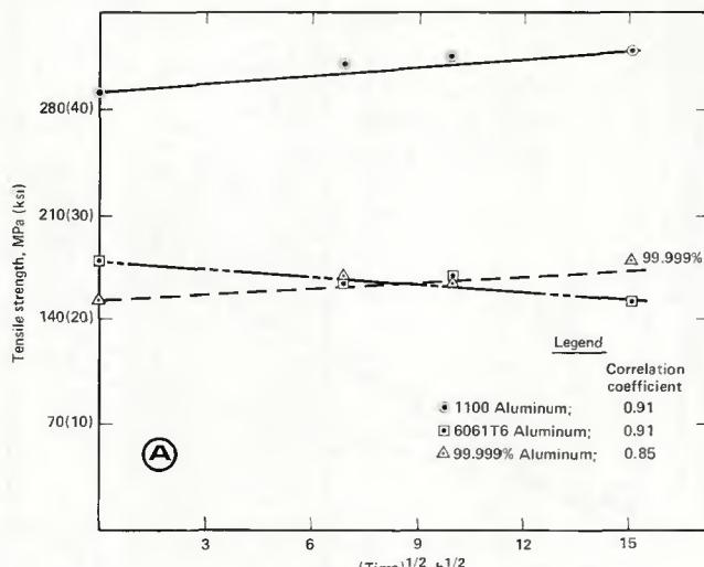
Fig. 3—The dependence of the weld strength on aging time: A— $T = 423\text{ K}$ ; B— $T = 473\text{ K}$ ; C— $T = 513\text{ K}$
