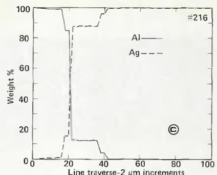
Fig. 8—Linear concentration profiles at a silver/aluminum or aluminum alloy weld interface. Specimens aged at 513 K for 49 h: A—pure aluminum; B—6061 aluminum alloy; C—6061 aluminum alloy
