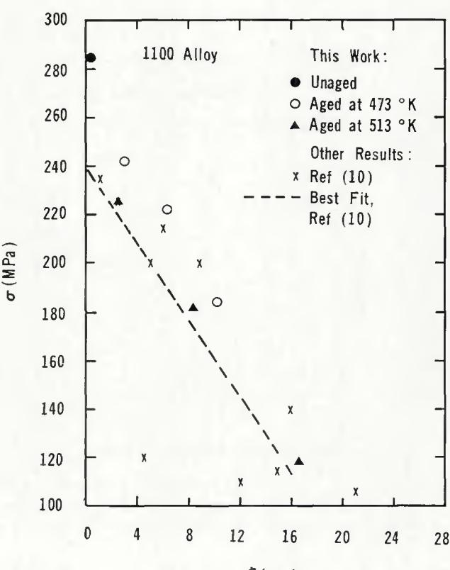
Fig. 10—The dependence of the strength of the weld between stainless steel and 1100 aluminum alloy on the total thickness of the intermetallic layer
