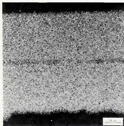
Fig. 6—Silver distribution at a stainless steel/6061 aluminum alloy weld aged at 513 K for 4 h. Dark line in the middle of this x-ray map is the consequence of voids
