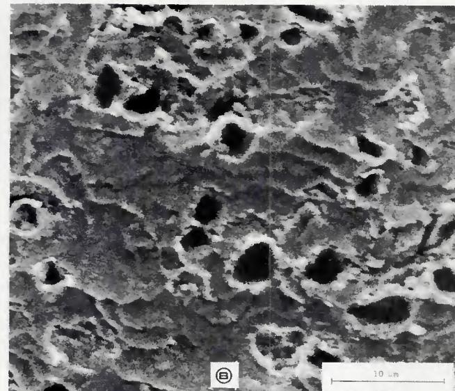
Fig. 14—Fracture surfaces of aged welds; specimens aged at 423 K for 225 h: A—between stainless steel and pure aluminum; B—between stainless steel and 1100 aluminum alloy
