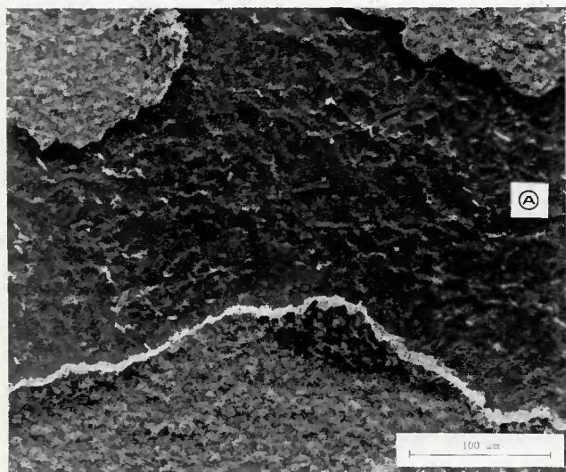
Fig. 13—Fracture surfaces of aged welds; specimens aged at 513 K for 49 h: A—between stainless steel and pure aluminum; B—between stainless steel and 1100 aluminum alloy
