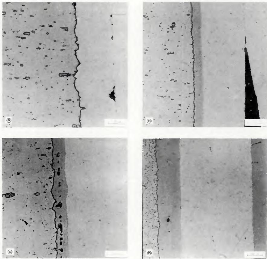
Fig. 1—Weld interface between stainless steel and 1100 aluminum alloy: A—unaged condition; B—after aging at 513 K for 4 h; C—after aging at 513 K for 16 h; D—after aging at 513 K for 49 h
