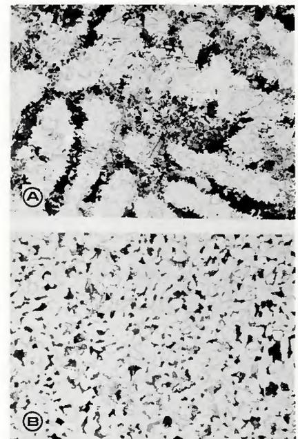
Fig. 13—As-cast and normalized heat 0 microstructures: A—as-cast; B—normalized. 2% nital etch, X250 (reduced 44% on reproduction)
