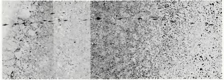
Fig. 14—Microstructure of 5 s stationary repair weld in heat 0. Nital etch, X75 (reduced 42% on reproduction)
