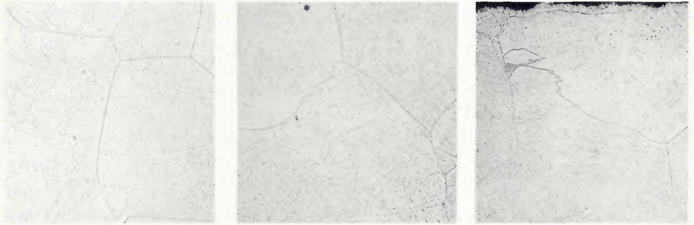
Fig. 16 - Comparison of microstructure revealed by OD plastic replication and metallographic mount of boat sample for the superheater outlet header. Left - replicating technique; center - direct viewing; right - transverse view
