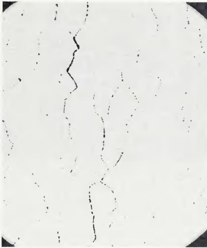
Fig. 5—Damage adjacent to main crack consisting of cavities and single grain facet (sgf) cracks (Unetched)
