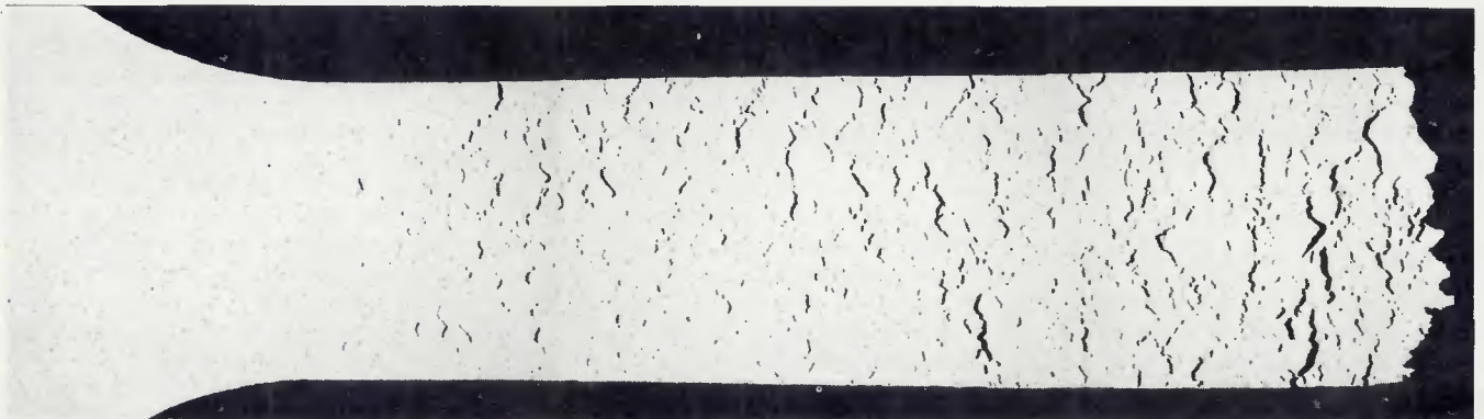
Fig. 14—Collage of creep specimen from 2B steam line. Specimen fractured at 750°C (1382°F) and 47 MPa (6.8 ksi)
