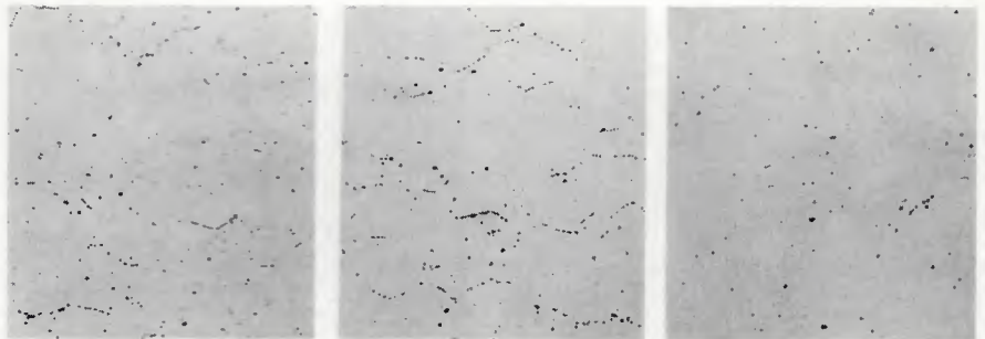
Fig. 6—Oriented cavitation in OD and midwall position while ID region is undamaged
