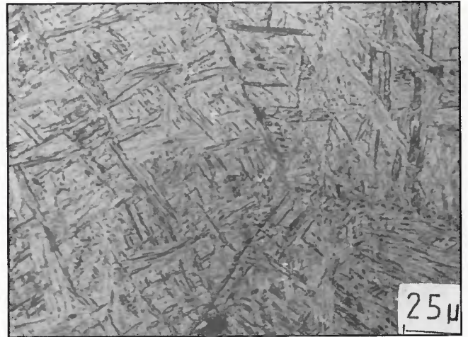
Fig. 4 — Fusion zone microstructure of Sample A.
