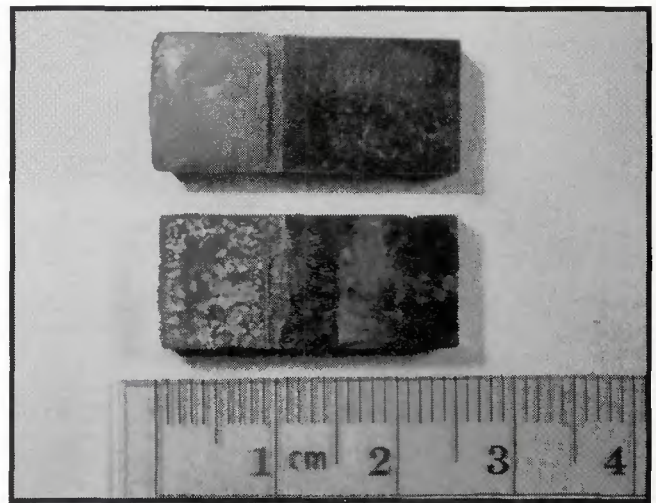
Fig. 11 — Fracture surfaces from shear tested joints brazed with 30Au-34Pd-36Ni (top) and 60Pd-40Ni.
