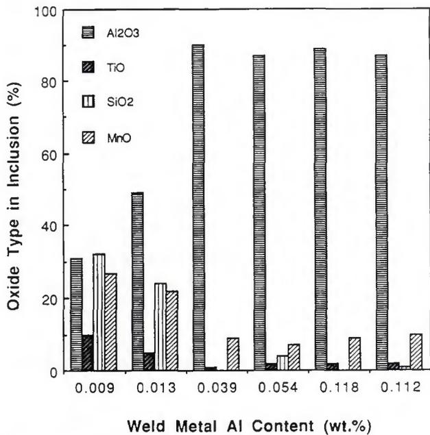
Fig. 12—Effect of weld metal aluminum content on inclusion composition.
