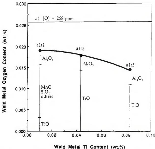
Fig. 14—Variation of weld metal oxygen content as a function of titanium additions in the aluminum-titanium group welds.
