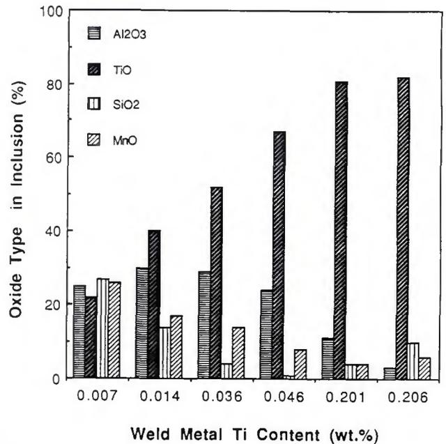
Fig. 13—Effect of weld metal titanium content on inclusion composition.
