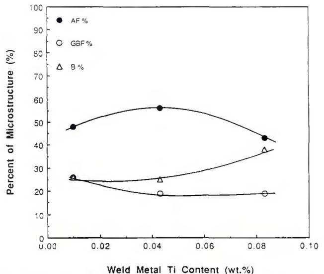
Fig. 15—Variation of weld metal microstructure as a function of titanium additions in the aluminum-titanium group welds.
