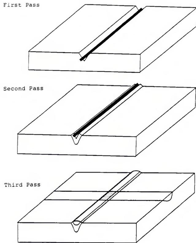
Fig. 2—Schematic drawing of the welding sequence.
