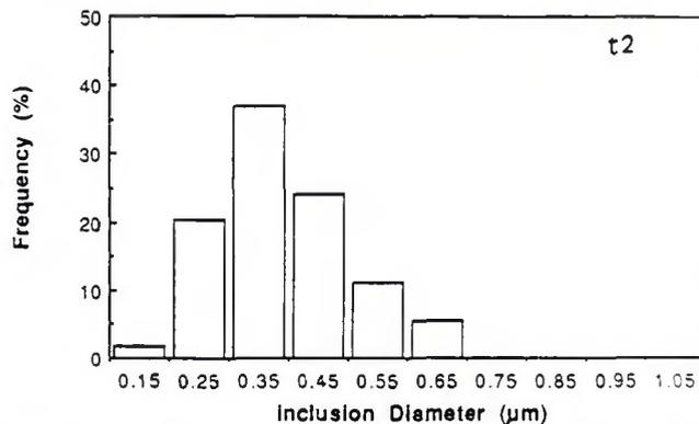
Fig. 10—Simple size distribution of the inclusions extracted from: A—Specimen t3 (Ti = 0.036 wt-%; Al = 0.009 wt-%; B—Specimen t2 (Ti = 0.014 wt-%; Al = 0.007 wt-%) with only titanium addition.
