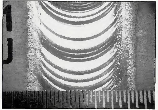
Fig. 10 — A — Weld front surface of pure cover pass. 8X magnification. Ruler divisions:  $\frac{1}{4}$  in. (0.4 mm); B — weld front surface of 100 ppm hydrogen in arc cover pass. Note severe ripples. 8X magnification. Ruler divisions:  $\frac{1}{4}$  in. (0.4 mm).
