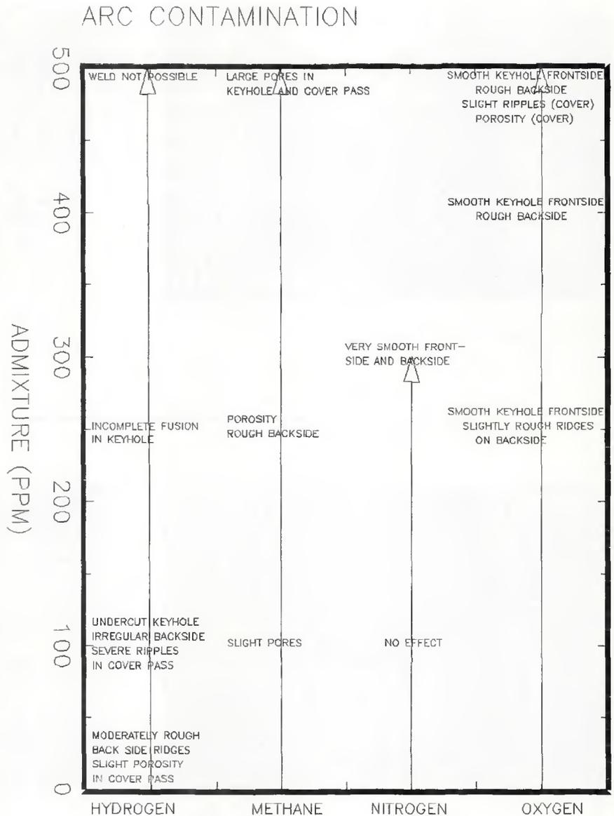
Fig. 4 — Chart shows the effects of arc gas contamination on the weld metal.
