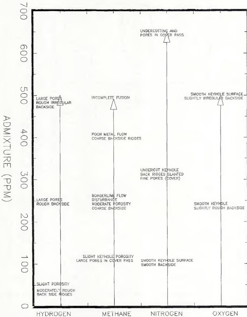
Fig. 3 — Chart shows the effects of shielding gas contamination on the weld metal.
