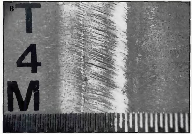
Fig. 13 — A — Weld backside of a pure gas with ridges perpendicular to weld direction. 8X magnification. Ruler divisions:  $\frac{1}{64}$  in. (0.4 mm); B — weld backside of 650 ppm nitrogen in shielding gas with ridges slanted toward undercut side. 8X magnification. Ruler divisions:  $\frac{1}{64}$  in. (0.4 mm).
