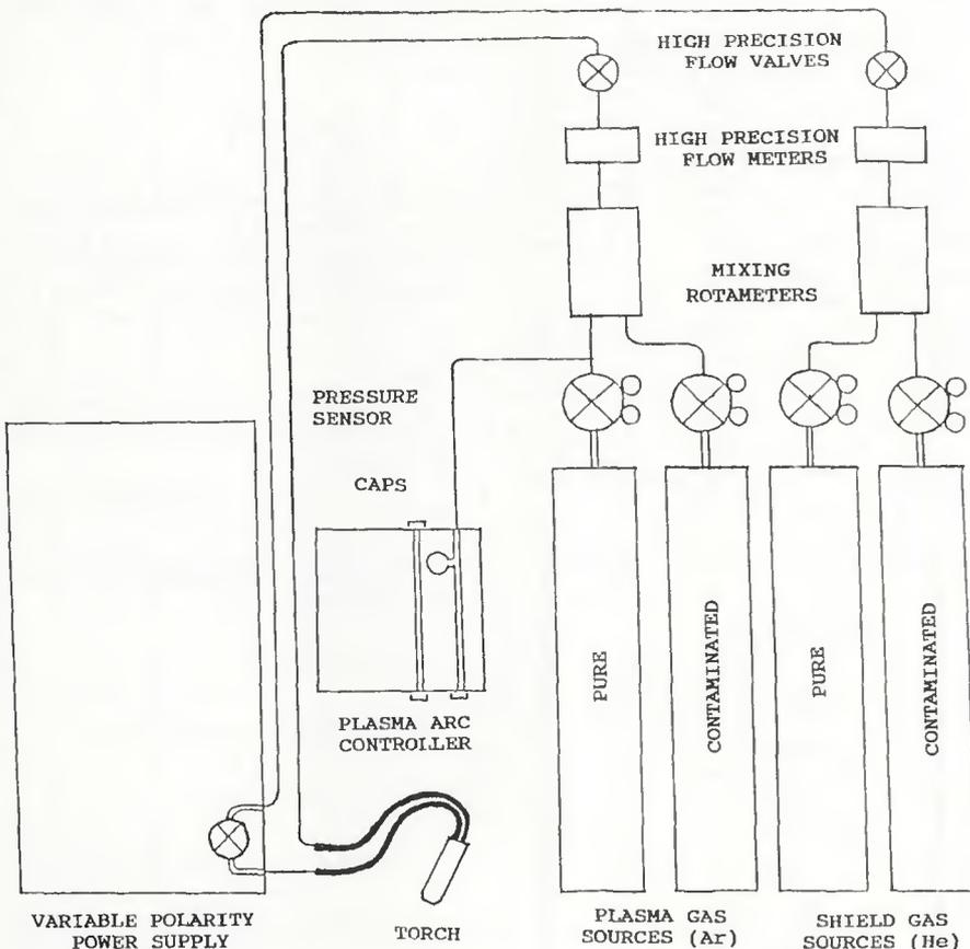
Fig. 1 — Schematic of experimental gas flow system.
