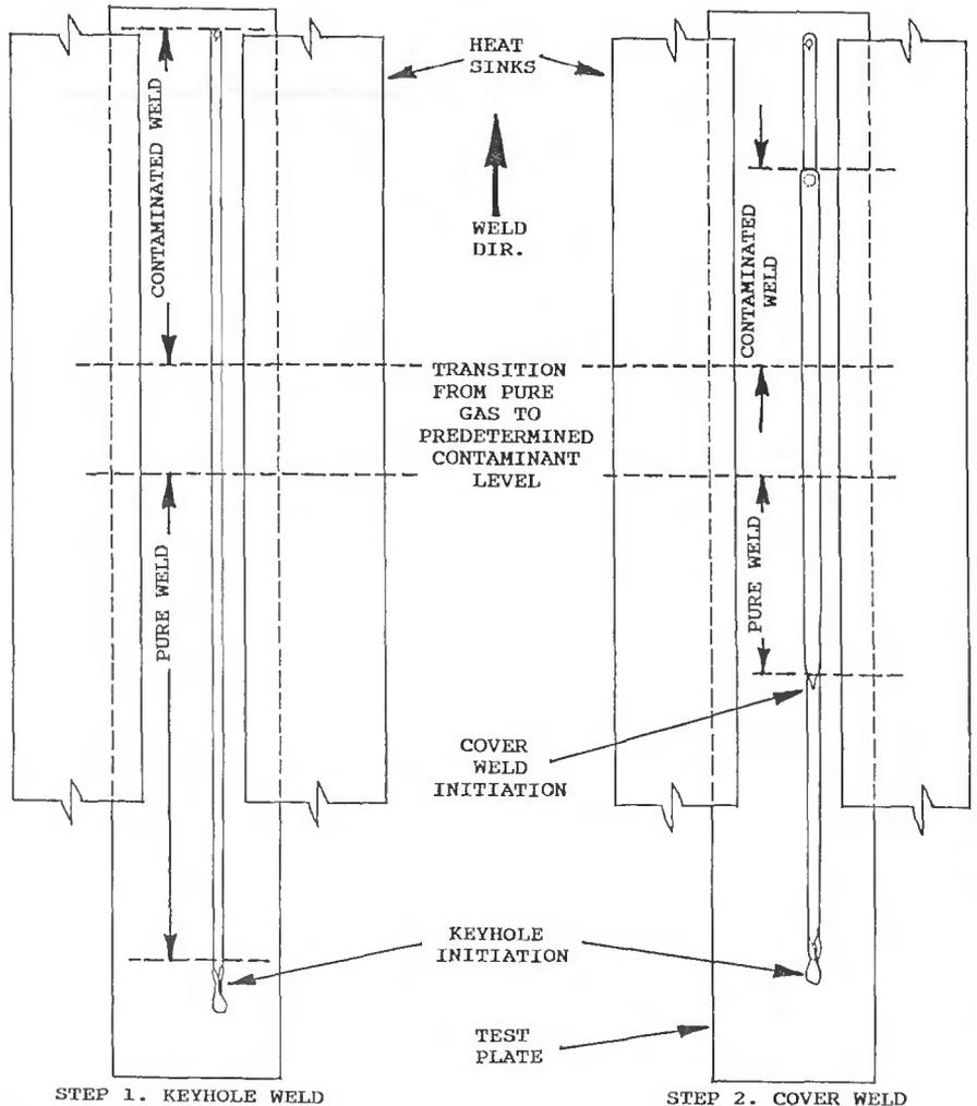
Fig. 2 — 2219 aluminum plate showing location of pure and contaminated welds and position of keyhole and cover passes.
