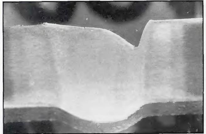
Fig. 8 — Weld cross-section of 400 ppm methane in shield showing poor fusion. 8X magnification.
