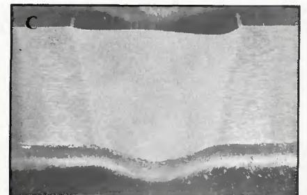
Fig. 12 — Weld cross-sections of 650 ppm nitrogen in shielding gas (B) and with pure gas (A, C). Note undercutting in contaminated section. 8X magnification.
