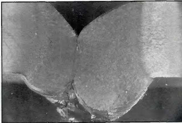
Fig. 7 — Weld cross-section of 250 ppm hydrogen in arc showing incomplete fusion. 8X magnification.
