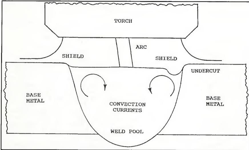
Fig. 11 — Schematic showing formation of weld undercut.
