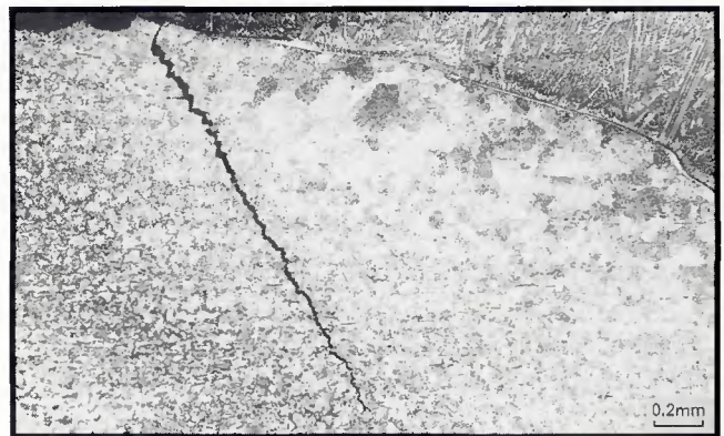
Fig. 5 — HAZ cracking from deposit toe, 50X.
