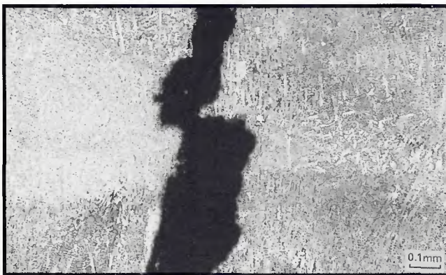
Fig. 4 — Typical deposit cracking, 100X.
