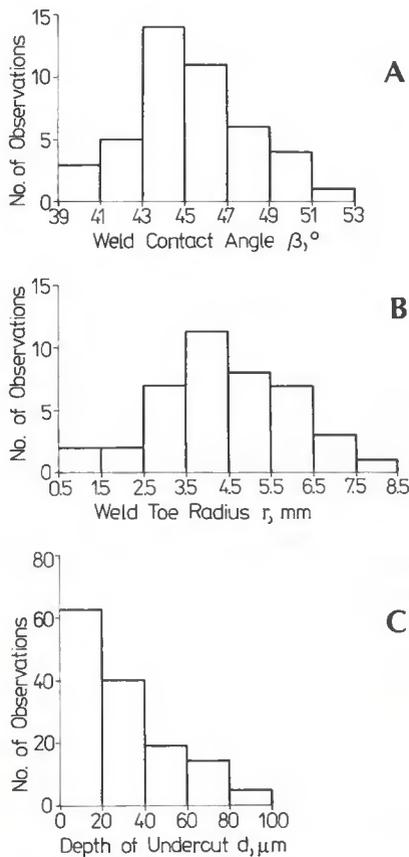
Fig. 3—Measured variations of geometry parameters for test specimens: A—Weld contact angle  $\beta$ , B—Root radius at the weld toe  $r$ ; C—Depth of undercut  $d$ .
