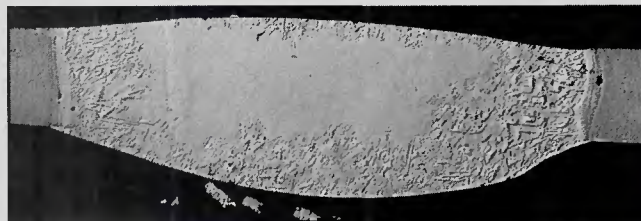
Fig. 17 — Weld made with preweld heat treatment at 750°F for 100 h in vacuum, DCEN, ER5356 (Alcoa etch: nitric, hydrofluoric, chromic acids; 11X).
