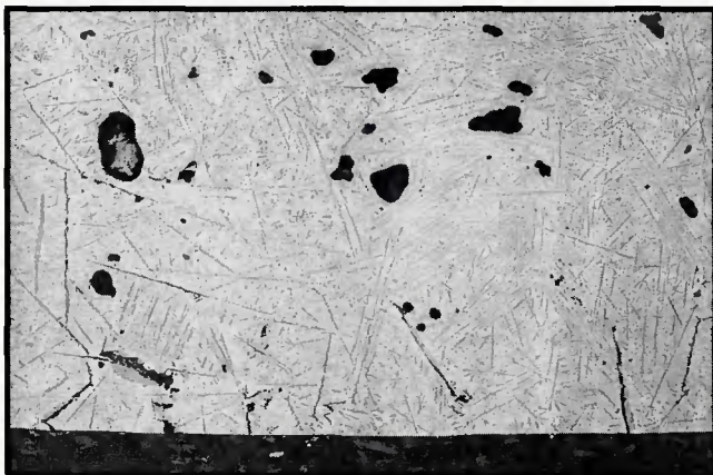
Fig. 8 — Top left: Microstructure of AC autogeneous weld at the weld toe area.
