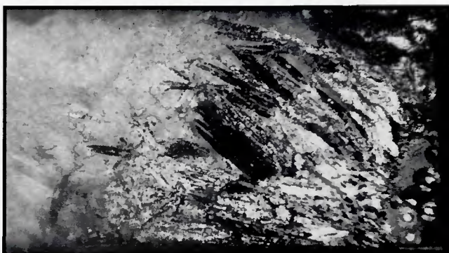
Fig. 21 — Massive and closely spaced acicular FeAl 3 on fracture surface of tension specimen with longitudinal weld (N465) (32X).
