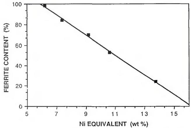
Fig. 6 — Relation between nickel equivalent and ferrite content measured using point counting.
