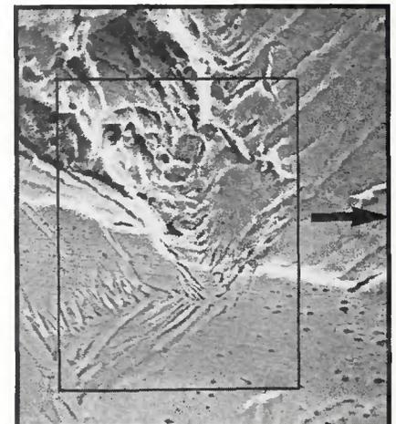
Fig. 13 — Correspondence between the ductile tear region on the fracture surface of a broken WM-SERT test specimen and the austenite plates in the weld metal microstructure. Specimen W-3 containing 70% ferrite. Magnification 1467X.
