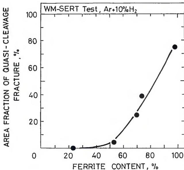
Fig. 10 — Relation between the area fraction of quasi-cleavage fracture on WM-SERT test specimens and ferrite content in duplex stainless steel weld metal.
