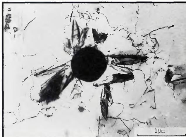
Fig. 16 — Cr<sub>2</sub>N precipitates nucleated by oxide inclusions in the weld metal.
