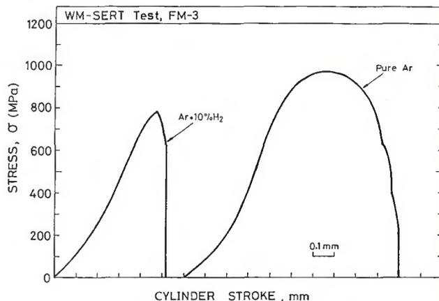
Fig. 4 — Applied stress/cylinder stroke relations during WM-SERT testing when using Ar and Ar-H<sub>2</sub> shielding gases. Weld metal W-3 containing 70% ferrite.
