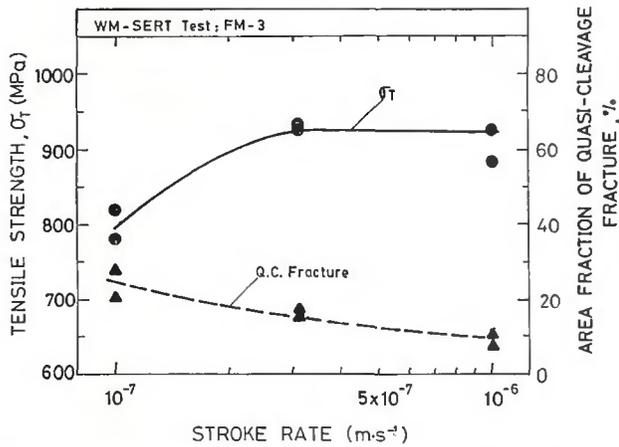
Fig. 5 — Effect of stroke rate on the peak tensile stress during WM-SERT testing ( $\sigma_T$ ), and on the area fraction of quasi-cleavage failure. Weld metal W-3 containing 70% ferrite.
