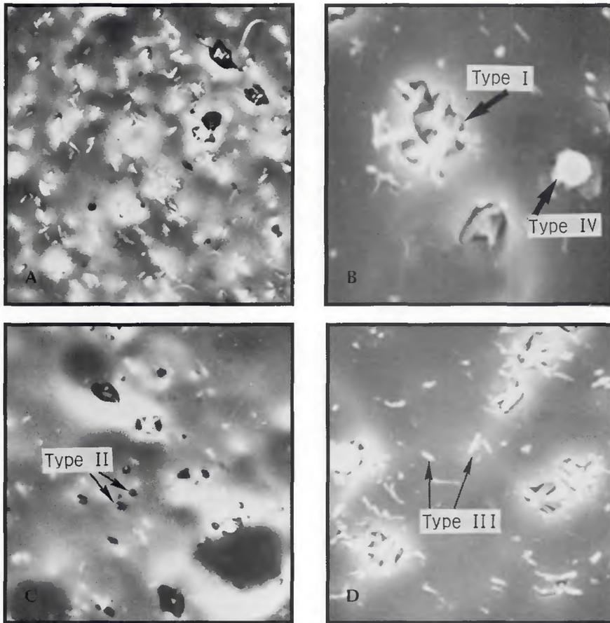
Fig. 14 — Modes of precipitation in weld metal containing 98% ferrite. A — General view (5000X); B — Type I and Type IV precipitates (13750X); C — Type II precipitates (6880X); D — Type III precipitates (9167X).
