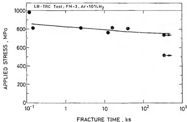
Fig. 2 — Relation between the applied stress and the time to fracture during LB-TRC testing. Weld metal W-3 containing 70% ferrite.
