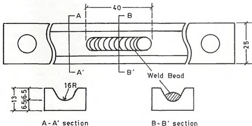
Fig. 1 — LB-TRC test configuration. B-B' indicates the slit prior to testing.
