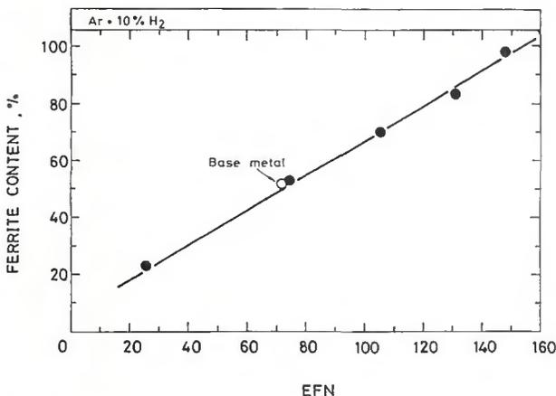
Fig. 7 — Relation between the extended ferrite number (FN) and the ferrite content found using point counting.
