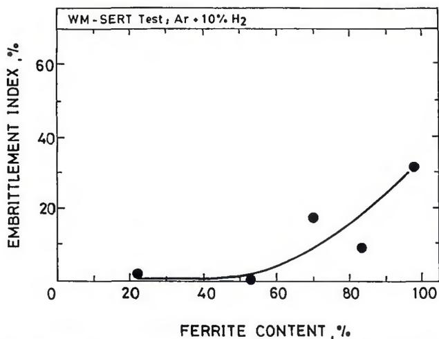
Fig. 9 — Effect of ferrite content on the hydrogen cracking susceptibility of duplex stainless steel weld metal. The embrittlement index is given as (NTS-LCS/NTS), where the NTS and LCS values are the test results produced using Ar and Ar-H<sub>2</sub> shielding gases.
