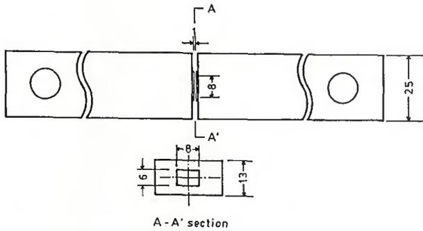
Fig. A-1 — The approximation used for analyzing weld zone dimensions during WM-SERT testing.
