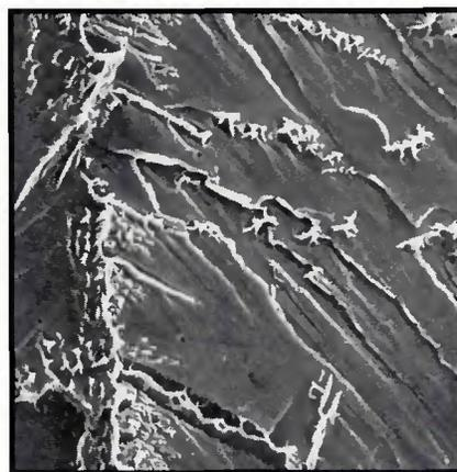
Fig. 3 — Fracture surface of an LB-TRC test specimen. Weld metal W-3 containing 70% ferrite.
