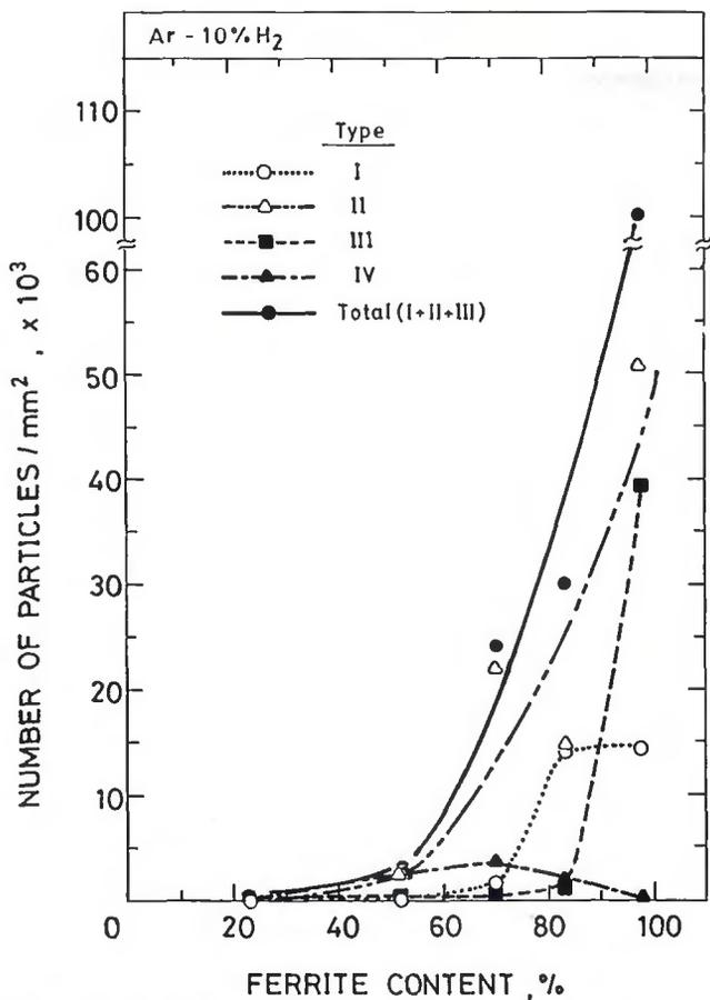
Fig. 15 — Relation between precipitation and ferrite content in the weld metal microstructure.
