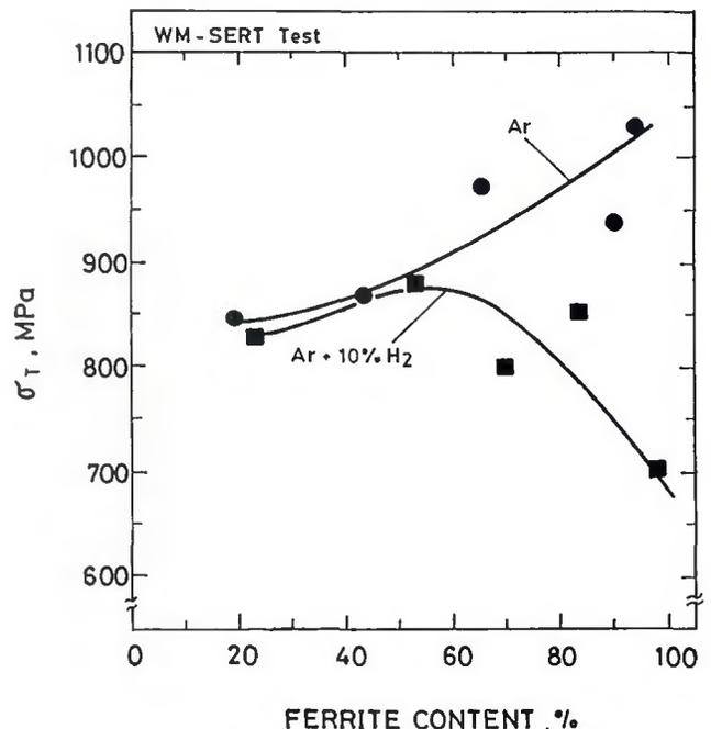
Fig. 8 — Effect of ferrite content on  $\sigma_T$  values when using Ar and Ar-H<sub>2</sub> shielding gases.
