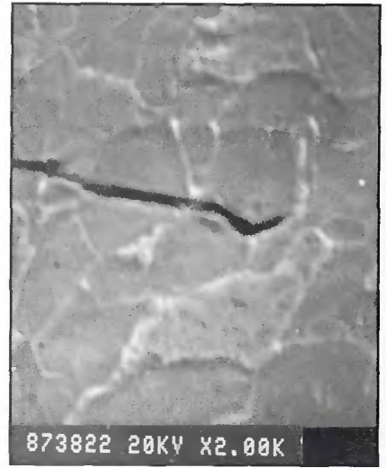
Fig. 11—The remaining crack in the impacted weld, 2000X.
