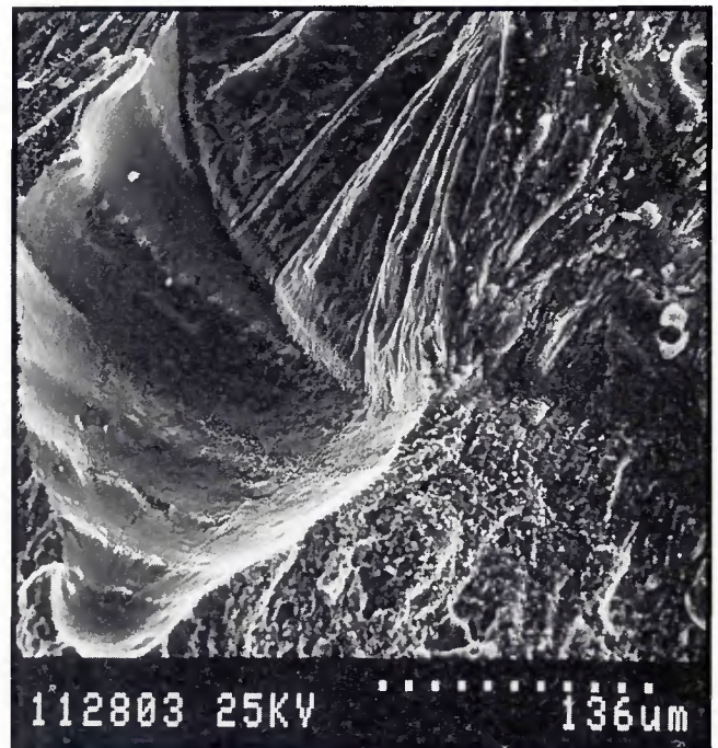
Fig. 5 — SEM fractograph of LDC weld showing: Left — Solidification patterns; right — pore growth over successive laser pulses.
