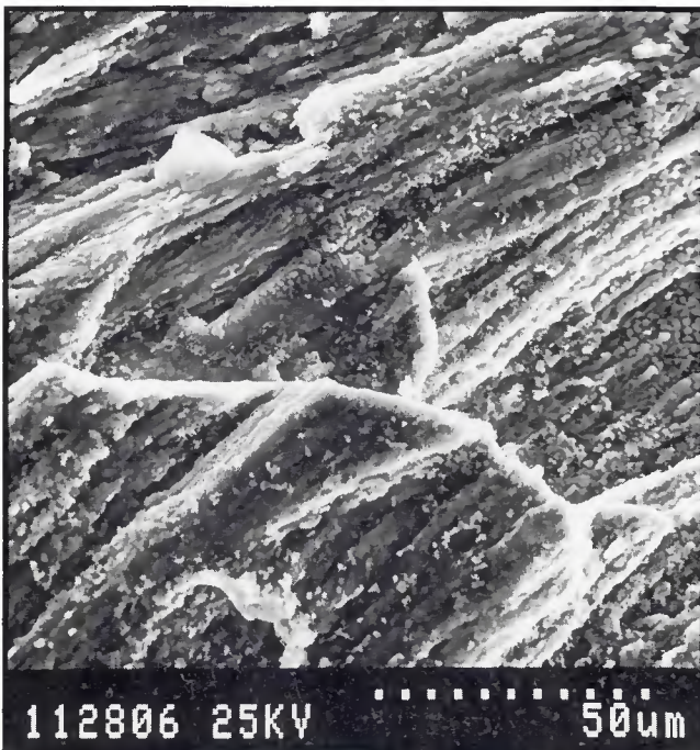
Fig. 5 — SEM fractograph of LDC weld showing: Left — Solidification patterns; right — pore growth over successive laser pulses.
