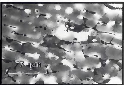
Fig. 8 — Bright field (BF) TEM images from HDC weld. A — Base material; B — heat-affected zone; C — fusion zone.
