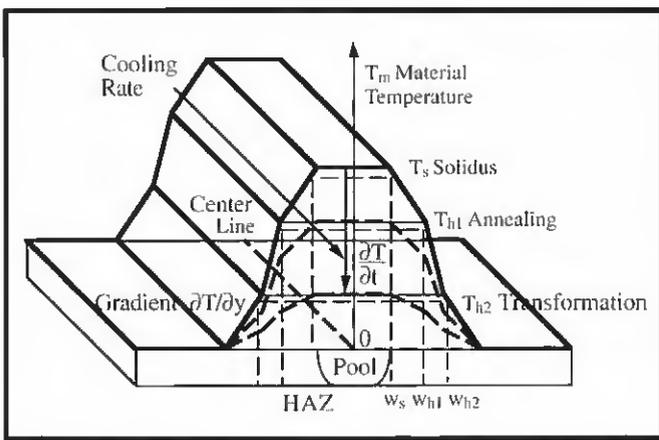
Fig. 9 — Specification of constitutive material temperature field  $T_m$ .
