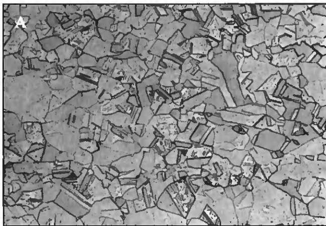
Fig. 6 — Microstructure of (A) as-received and (B) after 1300°C-peak thermal cycle for D2 composition (400X). Note virtual absence of particles of Nb compounds at grain boundaries.
