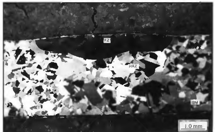
Fig. 10 — The shape of the fusion zone of Ni-270 (with Fe) GTA weld at 1 g.
