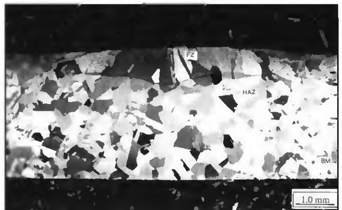
Fig. 12 — The shape of the fusion zone of Ni-270 (with Fe) GTA weld at 10 g.
