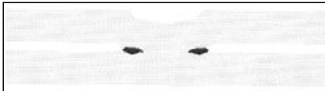
Fig. 8 — Predicted onset of expulsion at the end of the first half cycle using 8-kA welding current.
