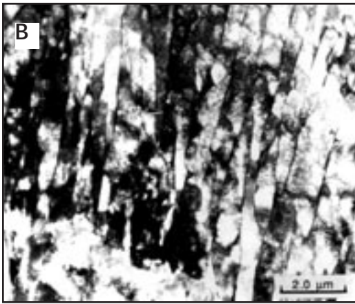
Fig. 5 — The microstructure of a large soft region in the fusion zone, in region 1 of Fig. 1C. A — Light micrograph; B — TEM micrograph of predominantly lath ferrite with some retained austenite (arrowed).
