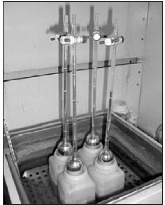
Fig. 3 — Eudiometer tubes and assembly for standard mercury displacement procedure.
