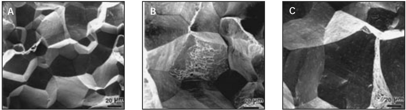
Fig. 9 — Scanning electron microscopy photomicrographs of fracture surfaces. Samples produced using an energy input of 2 kJ/mm and tested at a PWHT temperature of 675°C. A — HCM2S; B — 2.25Cr-1Mo tested at 325 MPa; C — 2.25Cr-1Mo tested at 270 MPa.
