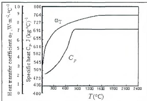
Fig. 7 — The heat transfer coefficient and specific heat vs. temperature.
