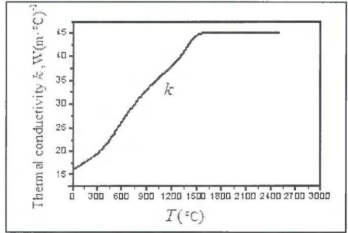
Fig. 6 — The thermal conductivity vs. temperature.
