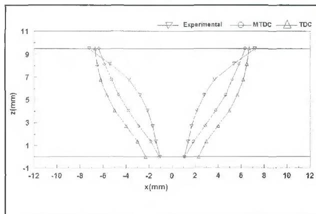
Fig. 8 — Comparison of predicted PAW cross section with experimental results.
