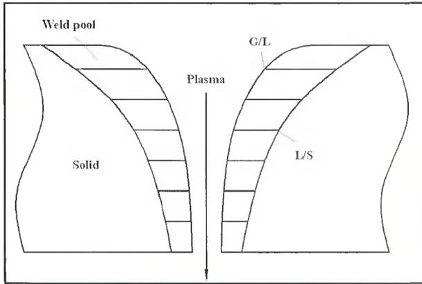
Fig. 3 — Schematic of keyhole and weld pool.
