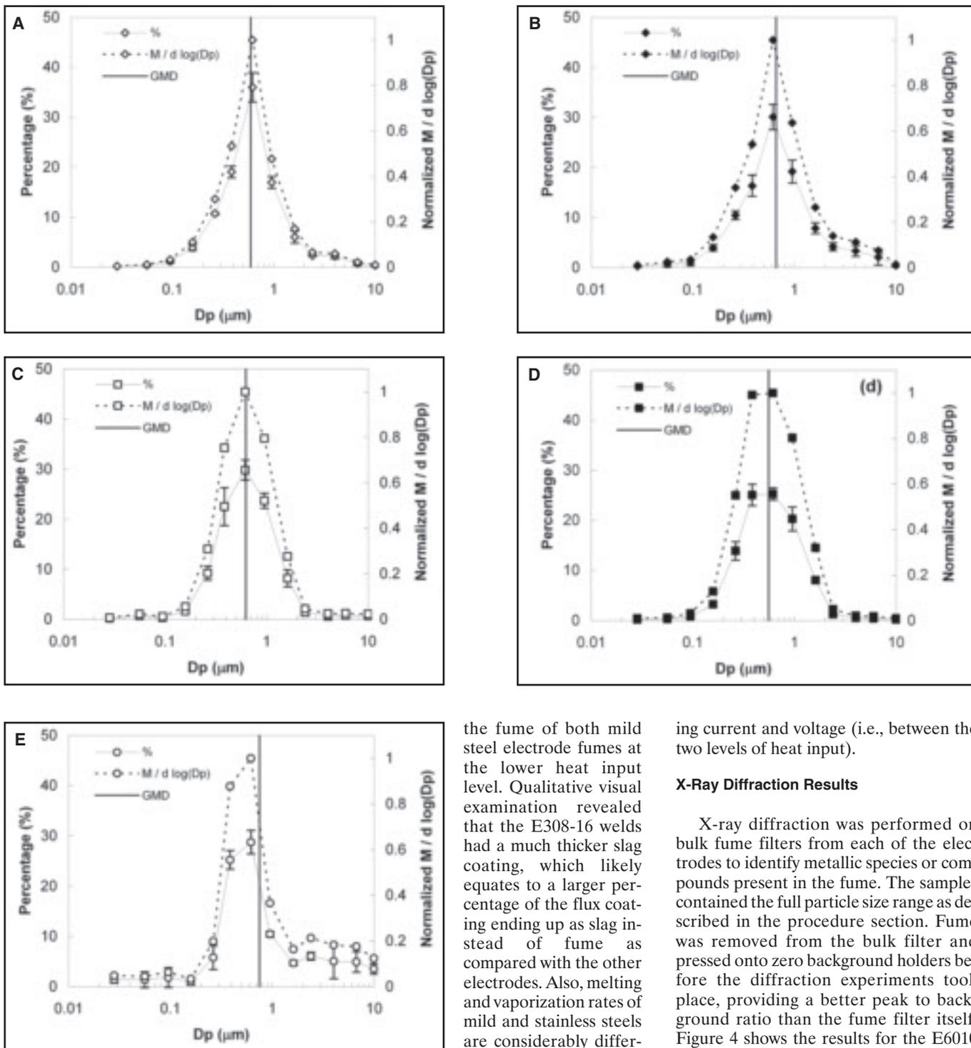
Fig. 8 — Particle mass distributions as a function of particle diameter for the following: A — E6010 low heat input; B — E6010 high heat input; C — E308-16 low heat input; D — E308-16 high heat input; E — E7018 nominal heat input. Vertical lines correspond to geometric mean diameter (GMD) of distributions.
