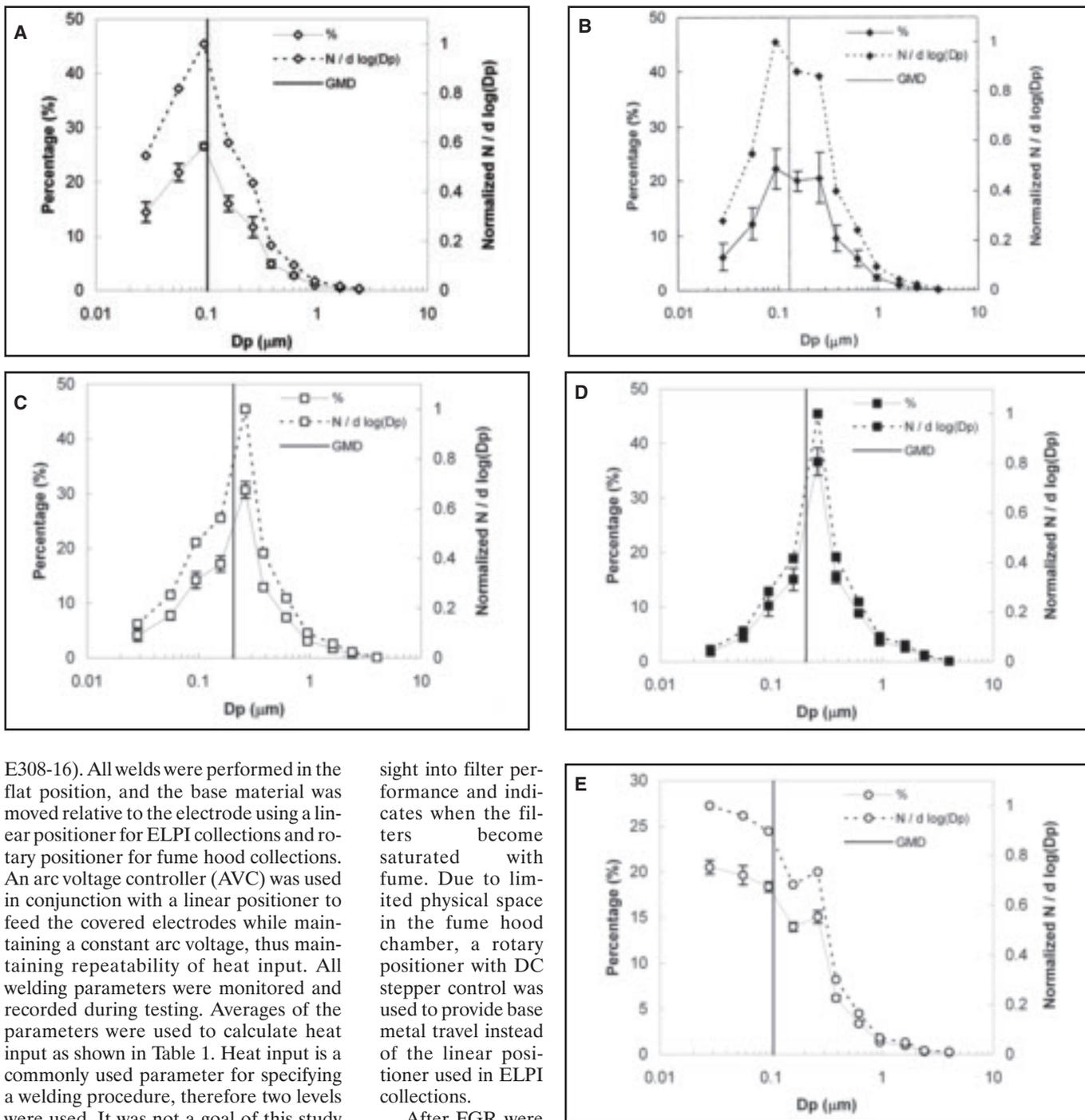
Fig. 7 — Particle number distributions as a function of particle diameter for the following: A — E6010 low heat input; B — E6010 high heat input; C — E308-16 low heat input; D — E308-16 high heat input; E — E7018 nominal heat input. Vertical lines correspond to geometric mean diameter (GMD) of distributions.
