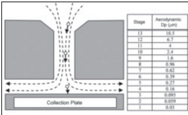
Fig. 1 — Principle of particle impact and aerodynamic cutoff size ranges of each ELPI stage (Ref. 24).
