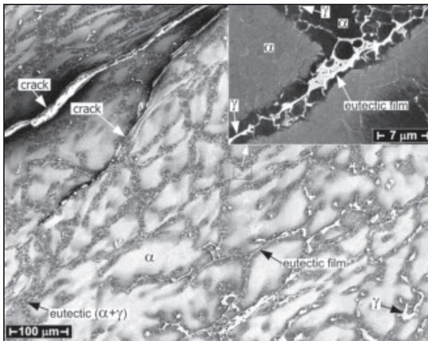
Fig. 7 — SEM image of weld of as-cast AZ91E Mg (small rectangle in Fig. 6B) showing evidence of eutectic liquid films during FSSW. Film enlarged in inset. 15-mm-diameter shoulder, 1000- rev/min rotation speed.
