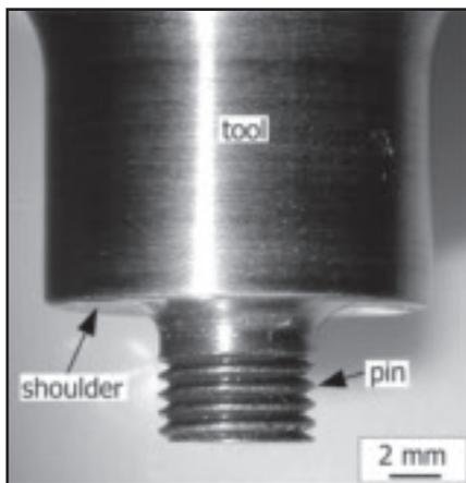
Fig. 2 — Tool with a 15-mm-diameter shoulder for FSSW with augmented torque (tool with a 10-mm-diameter shoulder not shown).
