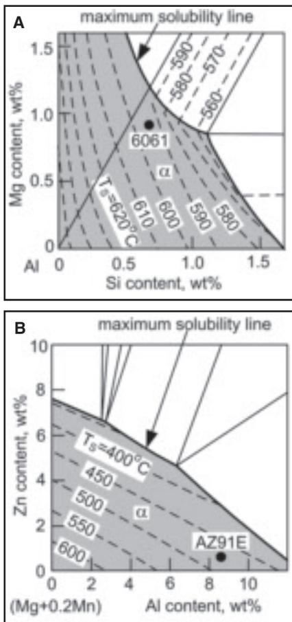
Fig. 13 — Solidus projections showing solidus temperature  $T_S$  and line of maximum solubility. A — Ternary Al-Mg-Si in Al ( $\alpha$ ) corner (Ref. 30); B — ternary (Mg+0.2Mn)-Al-Zn in (Mg+0.2Mn) corner (Ref. 21).
