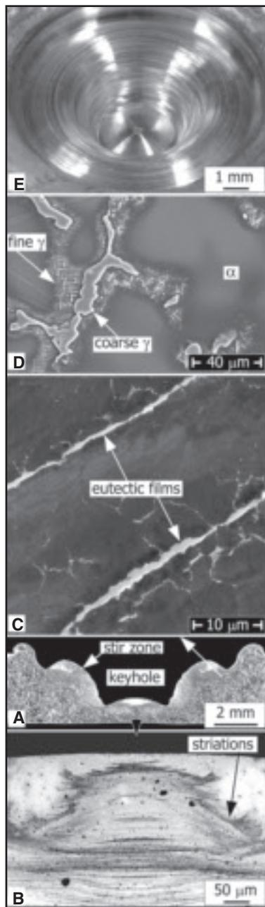
Fig. 3 — Liquation in weld of as-cast AZ91E Mg. A — Vertical cross section; B — optical micrograph showing striations below bottom of keyhole; C — SEM image showing evidence of liquid eutectic films; D — SEM image of base metal; E — weld surface. 10-mm-diameter shoulder, 1200-rev/min rotation speed.
