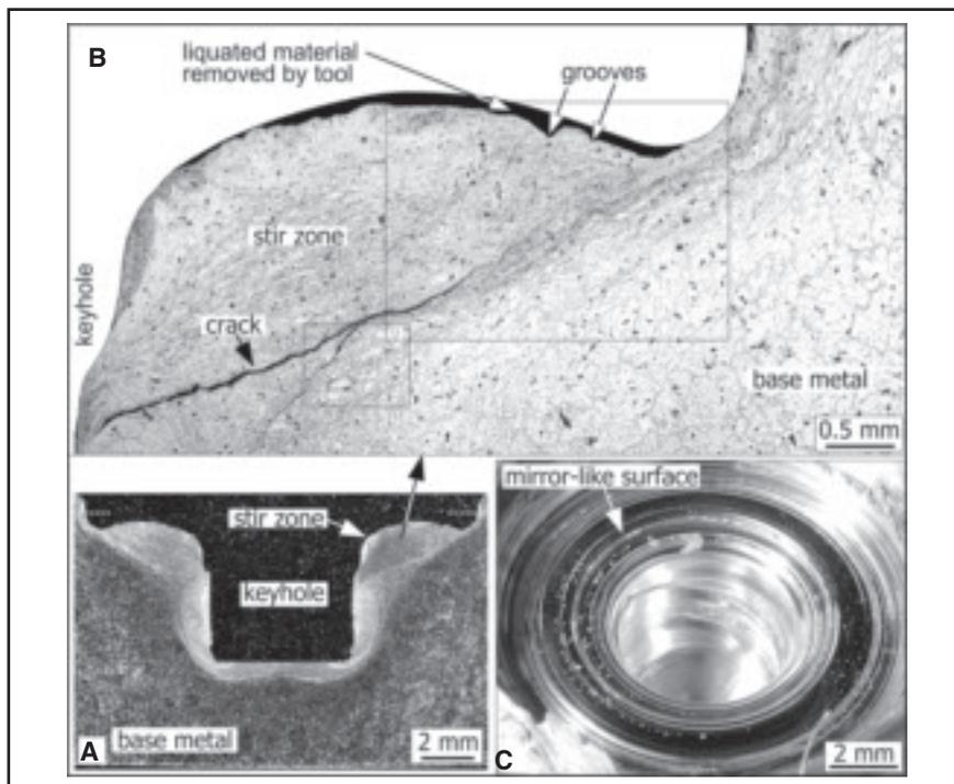
Fig. 6 — Liquation and cracking in weld of as-cast AZ91E Mg. A — Vertical cross section; B — evidence of liquation shown by cracking (small rectangle shown in Fig. 7 and large one Fig. 8A) and removal of liquated material by tool (black area at top of stir zone); C — evidence of liquation shown by mirror-like weld top surface. 15-mm-diameter shoulder, 100- rev/min rotation speed.
