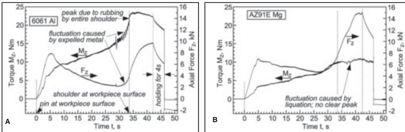
Fig. 11 — Tool torque and axial force measured during FSSW. A — 6061 Al; B — AZ91E Mg. Area under each curve proportional to heat input generated by either rotation ( $M_z$ ) or plunge ( $F_z$ ) of tool. 15-mm-diameter shoulder, 1000-rev/min rotation speed.
