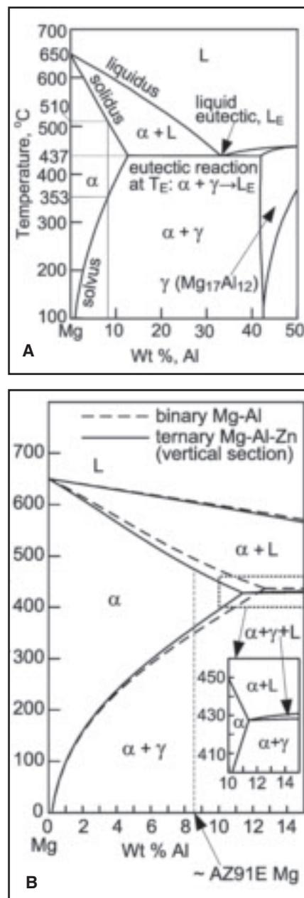
Fig. 9 — Mg phase diagrams. A — Binary Mg-Al phase diagram (Ref. 22); B — vertical section (solid lines, also called isopleth) of Mg-Al-Zn ternary phase diagram at Al/Zn = 8.60/0.65, with a binary Mg-Al phase diagram (broken lines) included for comparison. Both phase diagrams in B calculated using Pandat of CompuTherm LLC (Ref. 23) and Mg database (Ref. 24).
