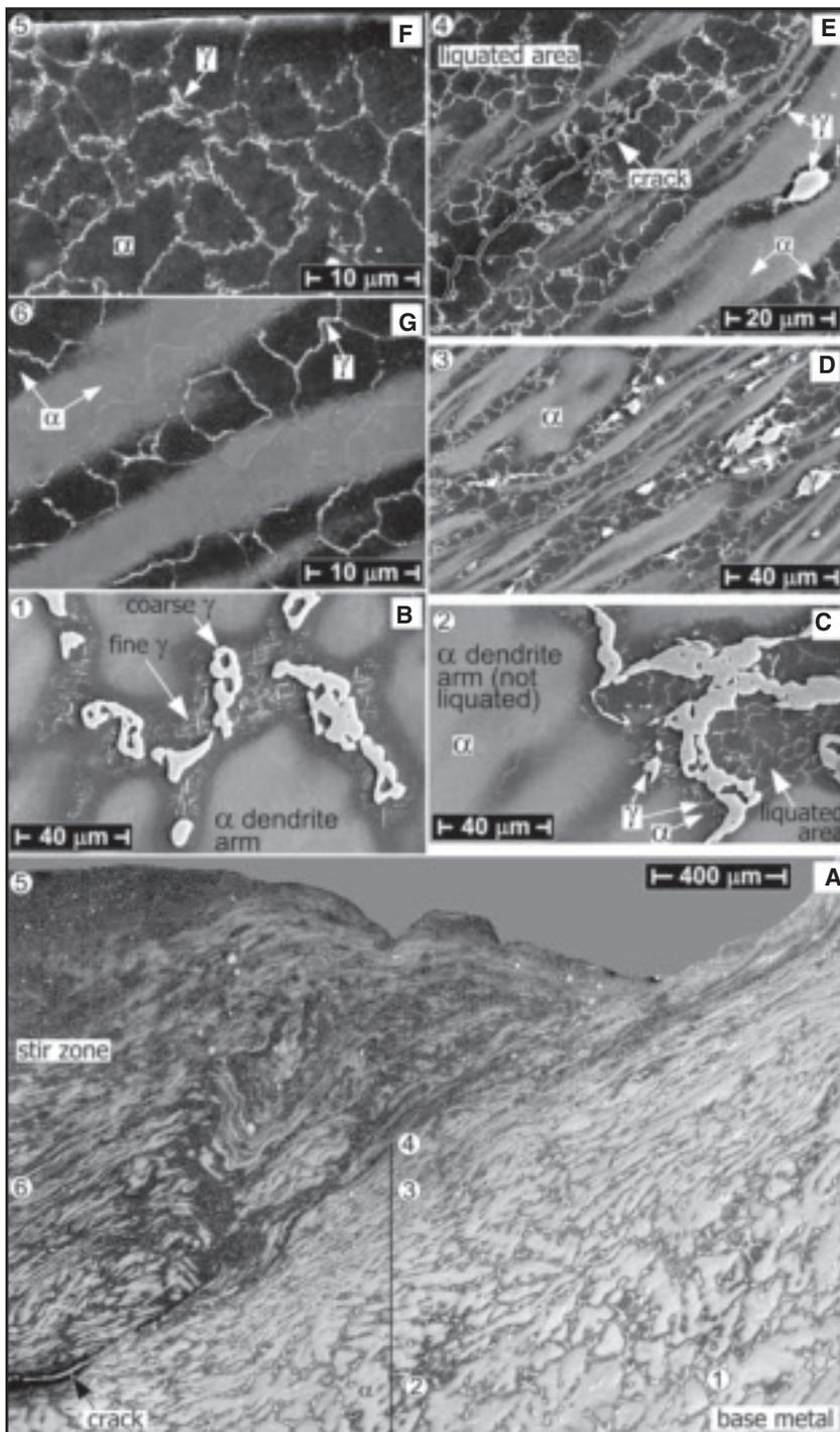
Fig. 8 — SEM images of weld of as-cast AZ91E Mg. A — Vertical cross section (large rectangle in Fig. 6B); B — base metal at point 1 in A; C — liquation at point 2; D — deformation and more liquation at point 3; E — cracking at point 4; F — liquation at point 5; G — liquation at Point 6. 15-mm-diameter shoulder, 1000-rev/min rotation speed.
