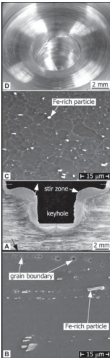
Fig. 5 — No liquation in weld of 6061-T6 Al. A — Vertical cross section; B — SEM image showing base metal microstructure; C — SEM image showing microstructure near weld surface; D — weld surface. 15-mm-diameter shoulder, 1000-rev/min rotation speed.
