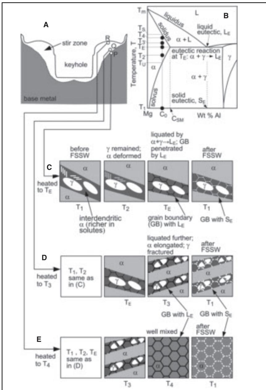
Fig. 10 — Microstructural evolution leading to liquation in FSSW of an alloy with a low eutectic temperature like most Mg alloys. A — Vertical weld cross section; B — phase diagram; C — point P in A (similar to Fig. 8C); D — point Q (similar to Fig. 8D); E — point R (similar to Fig. 8F). Recrystallized grain boundaries in  $\alpha$  dendrites (lighter  $\alpha$ ) not shown.
