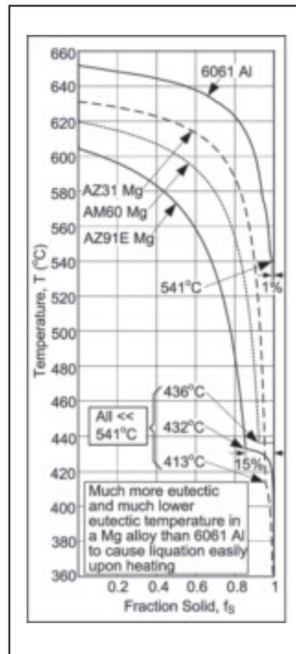
Fig. 12 —  $T-f_s$  curves during solidification explaining why Mg alloys are much more liquation susceptible than 6061 Al. Eutectic temperatures and contents: 541°C and 1% for 6061 Al, 432°C and 15% for AZ91E Mg, 436°C and 8% for AM60 Mg, and 413°C and 4% for AZ31 Mg. Curves calculated based on Scheil model of multicomponent alloys using Pandat of CompuTherm LLC (Refs. 21, 23).
