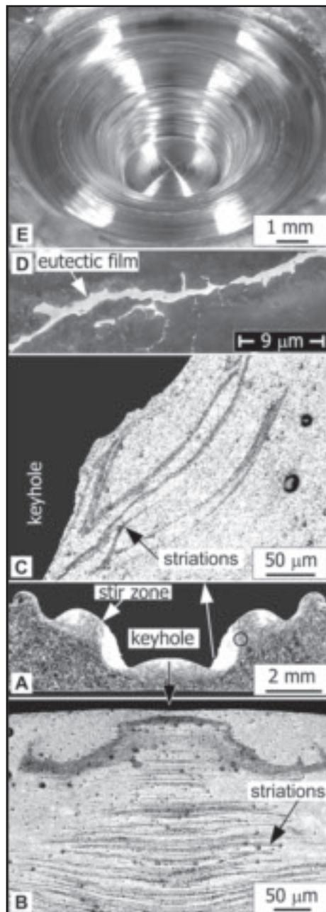
Fig. 4 — Liquation in weld of as-cast AZ91E Mg. A — Vertical cross section; B — optical micrograph showing striations below bottom of keyhole; C — optical micrograph showing striations around bottom of keyhole; D — SEM image showing eutectic film in the area circled in A; E — weld surface. 10-mm-diameter shoulder, 1000-rev/min rotation speed.
