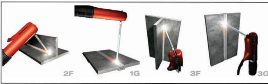
Fig. 2 — Images of weld types tested.
