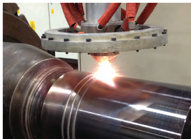
Fig. 2 — Laser cladding during the Bead 3 run.
