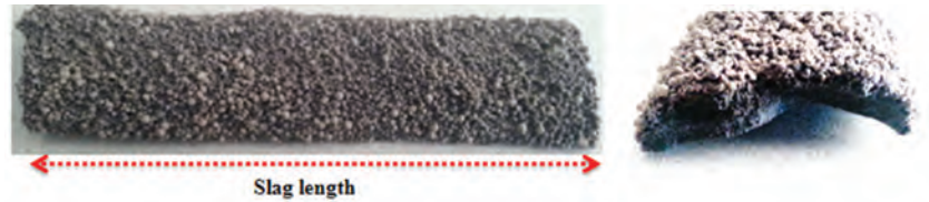
Fig. 3 — Solidified SAW slag.
