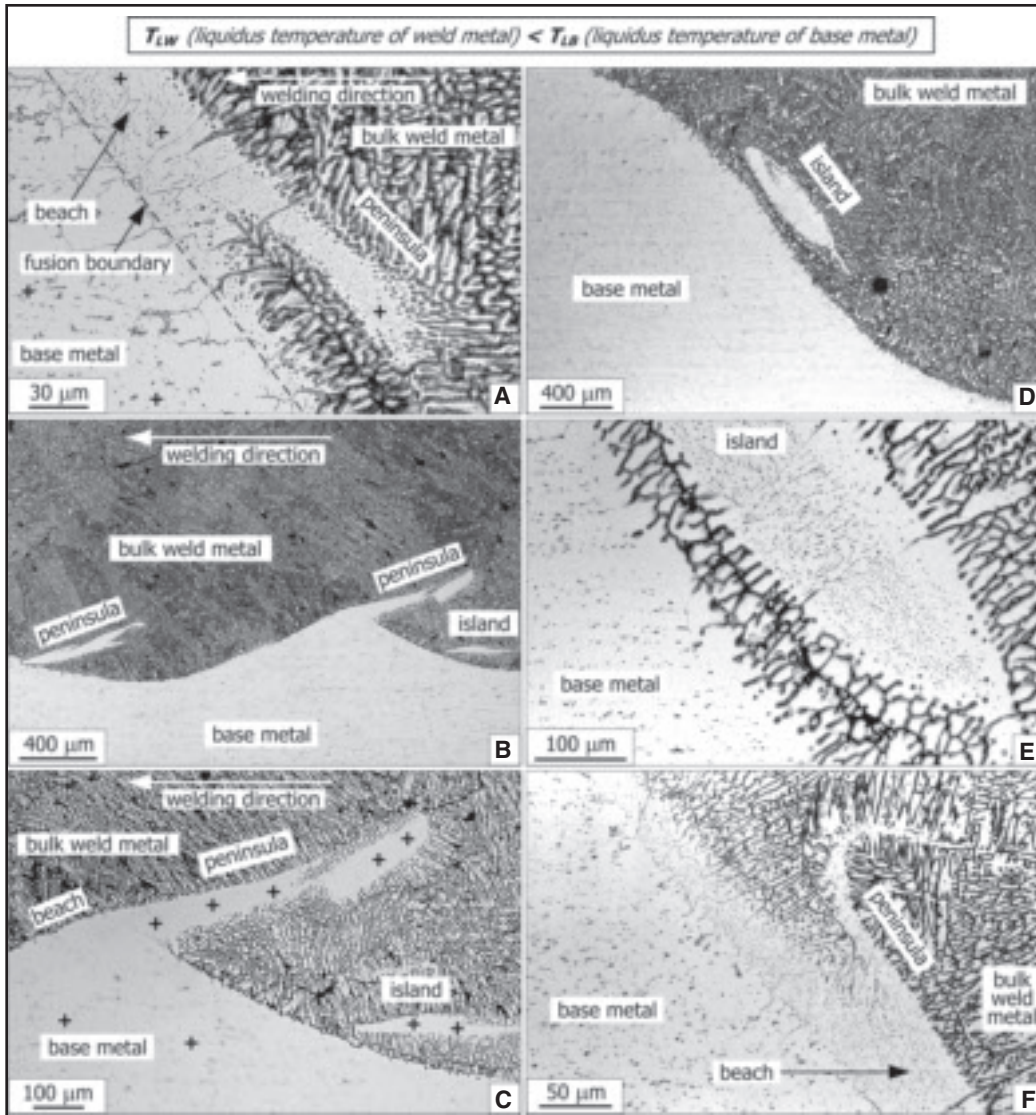
Fig. 4 — Filler-deficient beaches, islands, and peninsulas in gas metal arc welds of 1100 Al (pure Al) made with filler metal 4145 Al (Al-4Cu-10Si): A through C — Longitudinal micrographs (crosses indicate locations of composition measurements, which show neither Cu nor Si); D through F — transverse micrographs. (From Huang and Kou, Ref. 24.)
