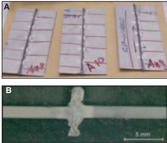
Fig. 2 — High-frequency welds made in advanced high-strength steels (different composition than the DP600 but still possessing near 600 MPa ultimate tensile strength). A — As-welded specimens; B — transverse micrograph. Previously published in Ref. 6. Used with permission from US Steel Research Europe, Kosice, Slovak Republic.
