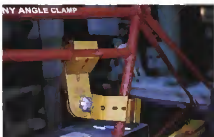
Fig. 13 — This lightweight aluminum clamp holds parts in place at a variety of angles.
