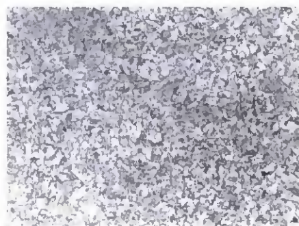
Fig. 4 — Microstructure of the API 5L X60 seamless pipe metal, austenitized at 920°C, water quenched, and tempered at 690°C.
