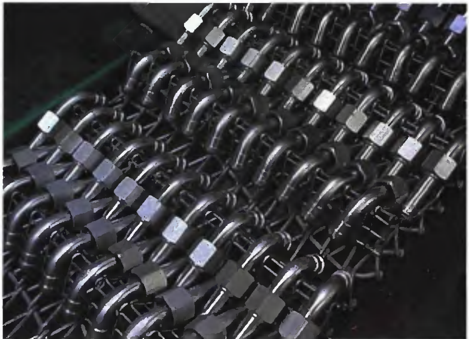
Fig. 7 — Bright-brazed AISI 304 stainless steel water pressure assemblies.
