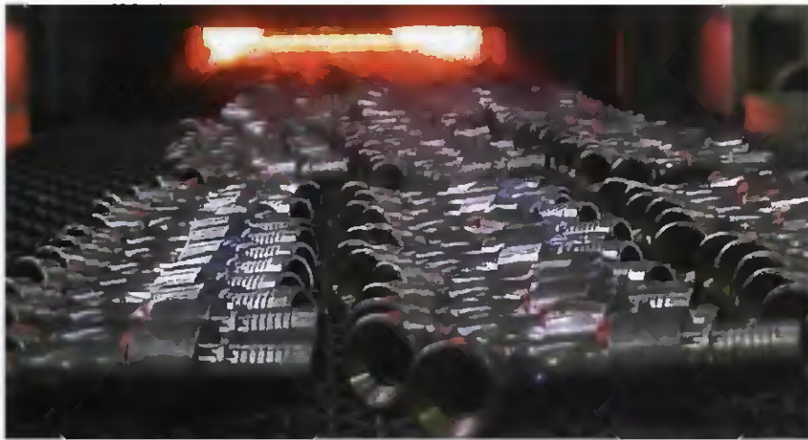
Fig. 3 — These self-jigging heavy elbow sections require a slow conveyor belt speed to braze properly.
