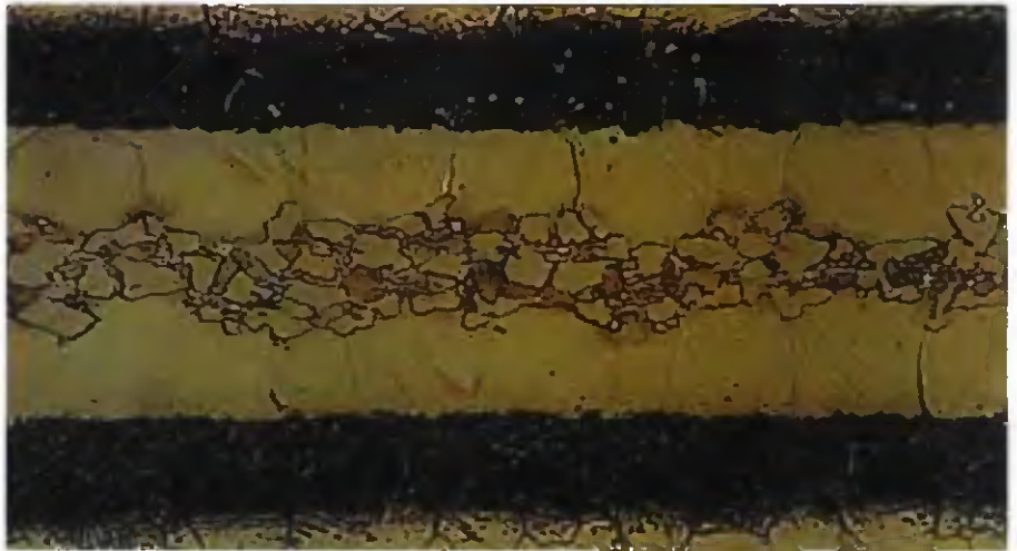
Fig 1 — Microphotograph of an etched 304L joint brazed with BNi-2.
