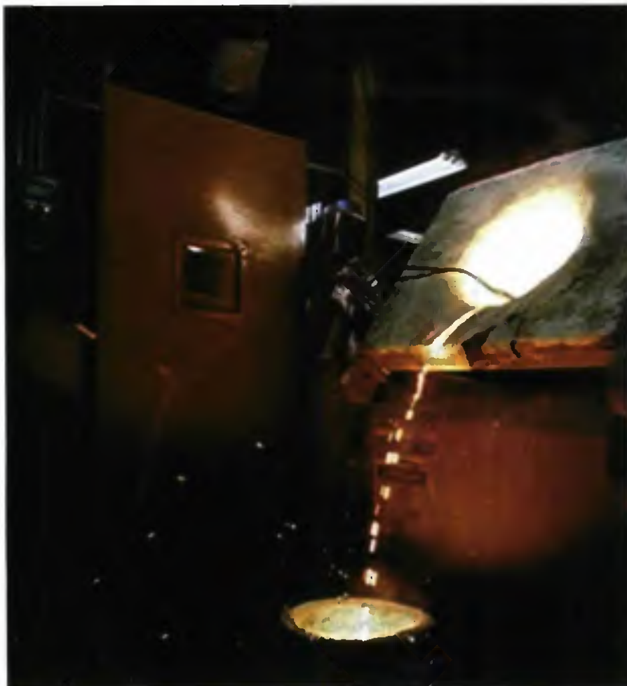
Fig. 3 — Refractory-lined furnace starting to pour the liquid metal for atomization.
