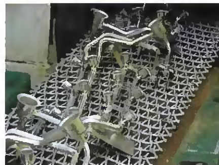
Fig. 2 — These AISI 304 stainless steel jigged fuel distributor A-pipes are brazed in pure hydrogen in a humpback furnace.
