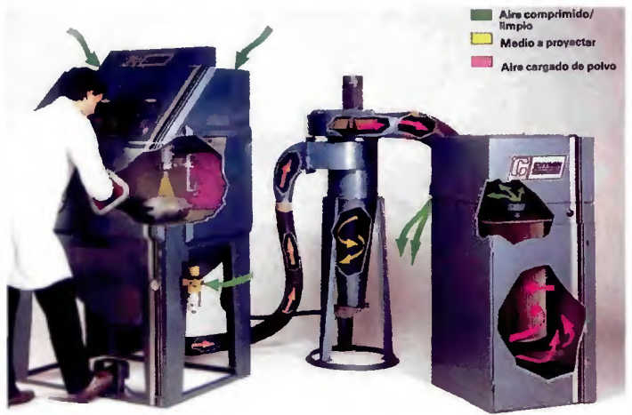
Fig. 2 — Cross sections of grit blast system units. (Courtesy of Guyson Corp., Saratoga Springs, N.Y.)
