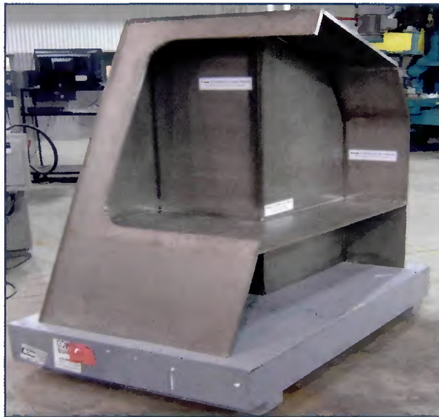
Fig. 1 — NJC built this complex titanium structure to evaluate a number of different joining processes that could be used to fabricate next-generation military combat vehicles.
