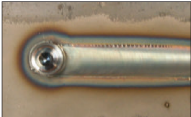
Fig. 7 — Appearance of a FS bead-on-plate weld in HSLA-65 with PCBN tool.
