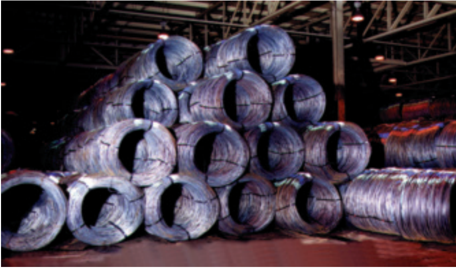
At Lincoln Electric, every coil of incoming rod (typically 2500 to 4500 lb of raw steel wire) is tested twice for chemical composition before it is put into production.
