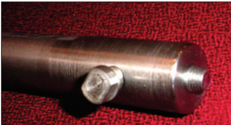
Fig. 5 — Photograph of two-piece refractory metal pin and shoulder assembly with locking screw.
