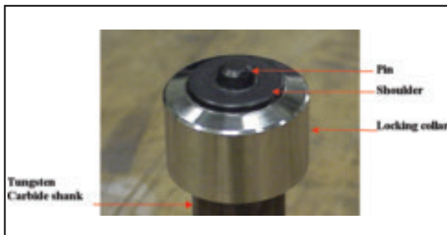
Fig. 2 — Details of PCBN tool used in FSW.
