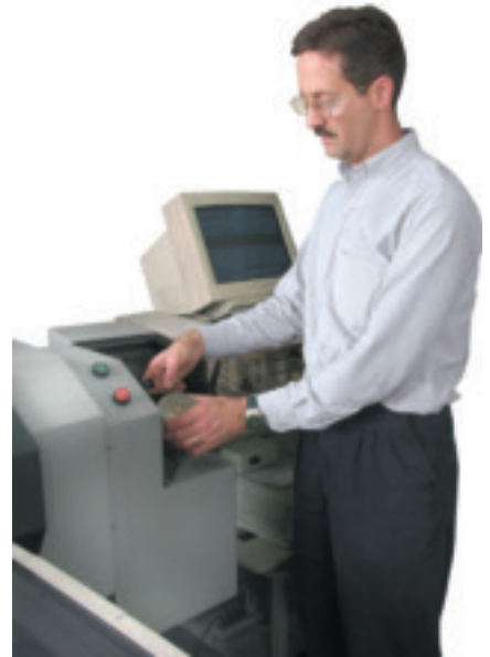
At Lincoln Electric, every coil of incoming rod (typically 2500 to 4500 lb of raw steel wire) is tested twice for chemical composition before it is put into production.
