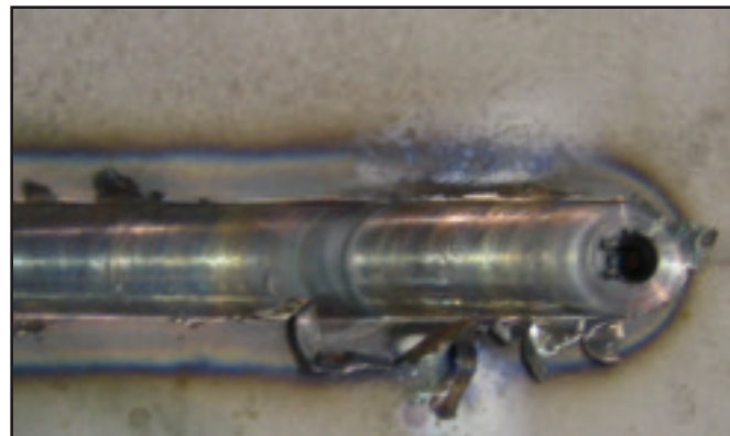
Fig. 8 — Appearance of weld surface in 0.25-in.- (6-mm-) thick HSLA-65 FSW weldment using W-Re tool.
