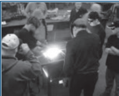
Gene Morrill demonstrated plasma arc cutting for the Spokane Section members.
