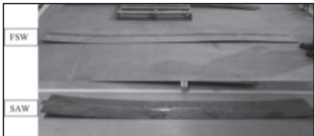
Fig. 9 — Completed 10-ft- (3-m-) long, 0.25-in.- (6-mm-) thick HSLA-65 weldments.
